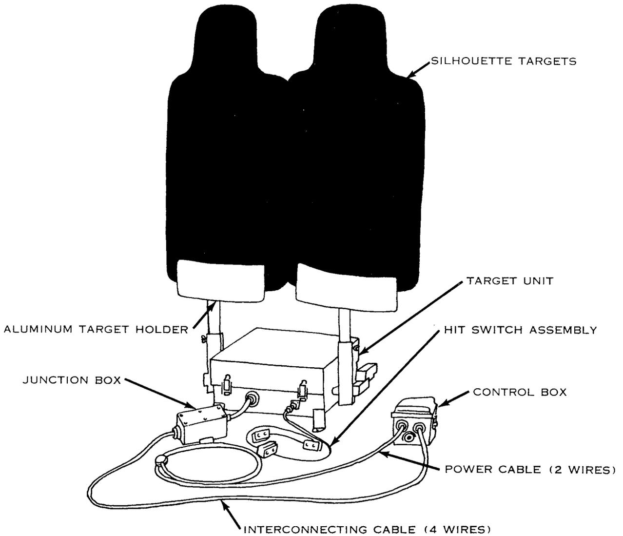
*Figure 98. Electrically controlled and scored pop-up target 3C52b.*
