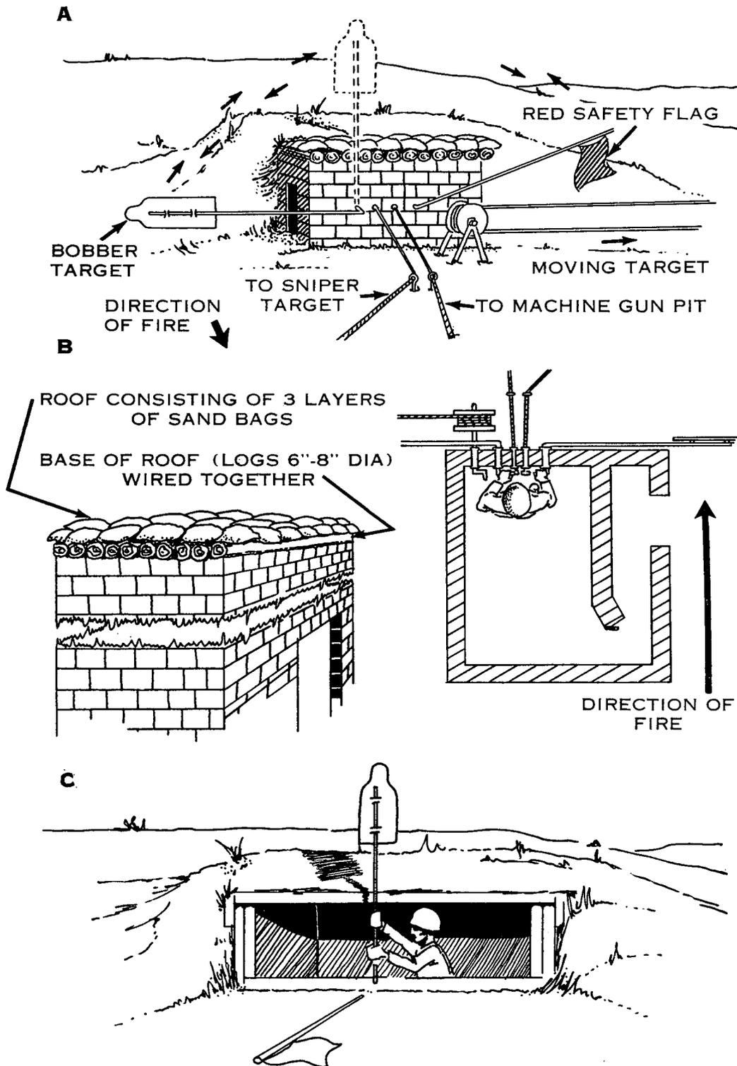
A—Outside view of a field target firing range personnel pit which must be used when grenade launchers are fired.
