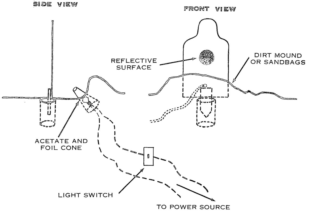
Figure 100. Flashing target device for night assault range.
