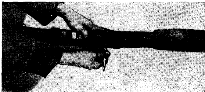
FIGURE 19.—To remove firing pin without disassembling rifle.
