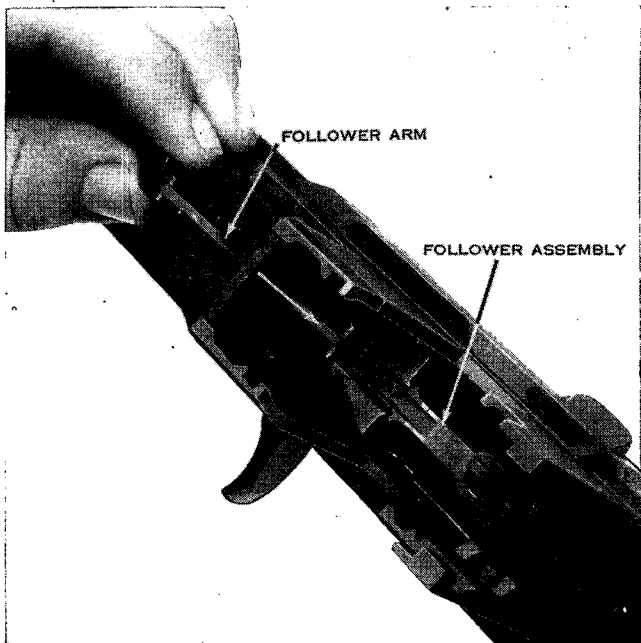
Figure 38. Replacing the follower arm.
