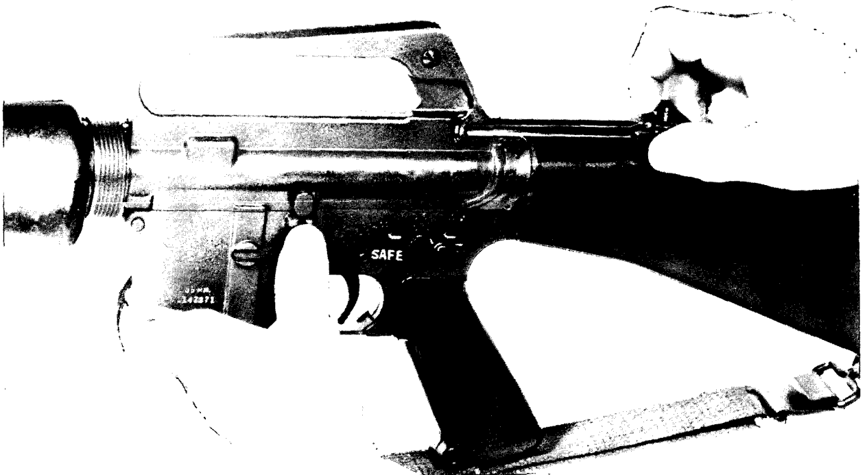
Figure 6. Locking the bolt open.
