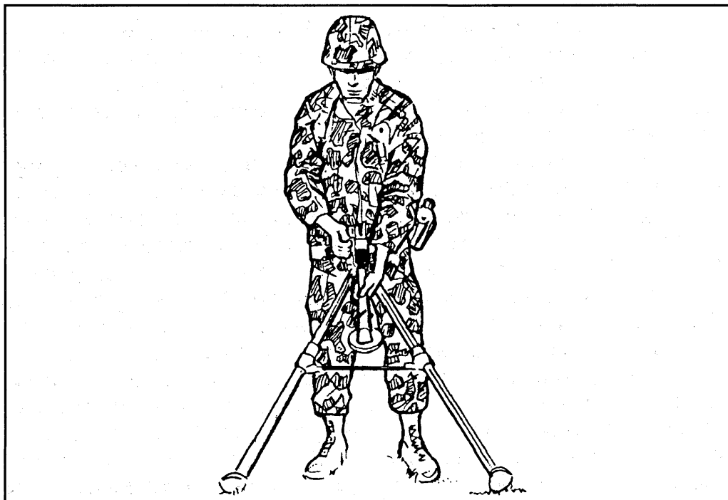
Figure 5-19. Emplacing the mount.
