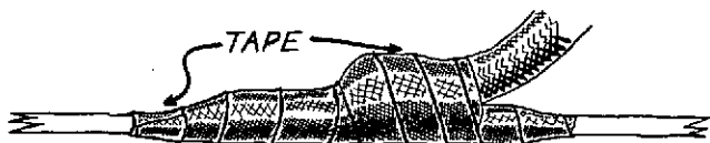
FIGURE 31.—Taping an insulated conductor spliced to bare wire.
