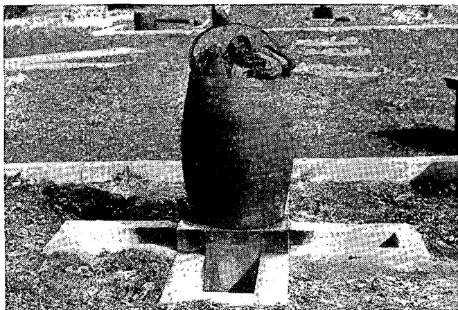
FIGURE 53.—Disinfestor, Serbian barrel type.
