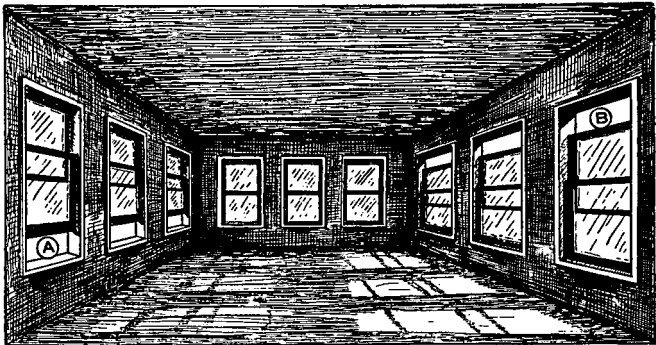
FIGURE 4.—Ventilation of squad rooms showing method of arranging window openings. A—Inlet. B—Outlet
