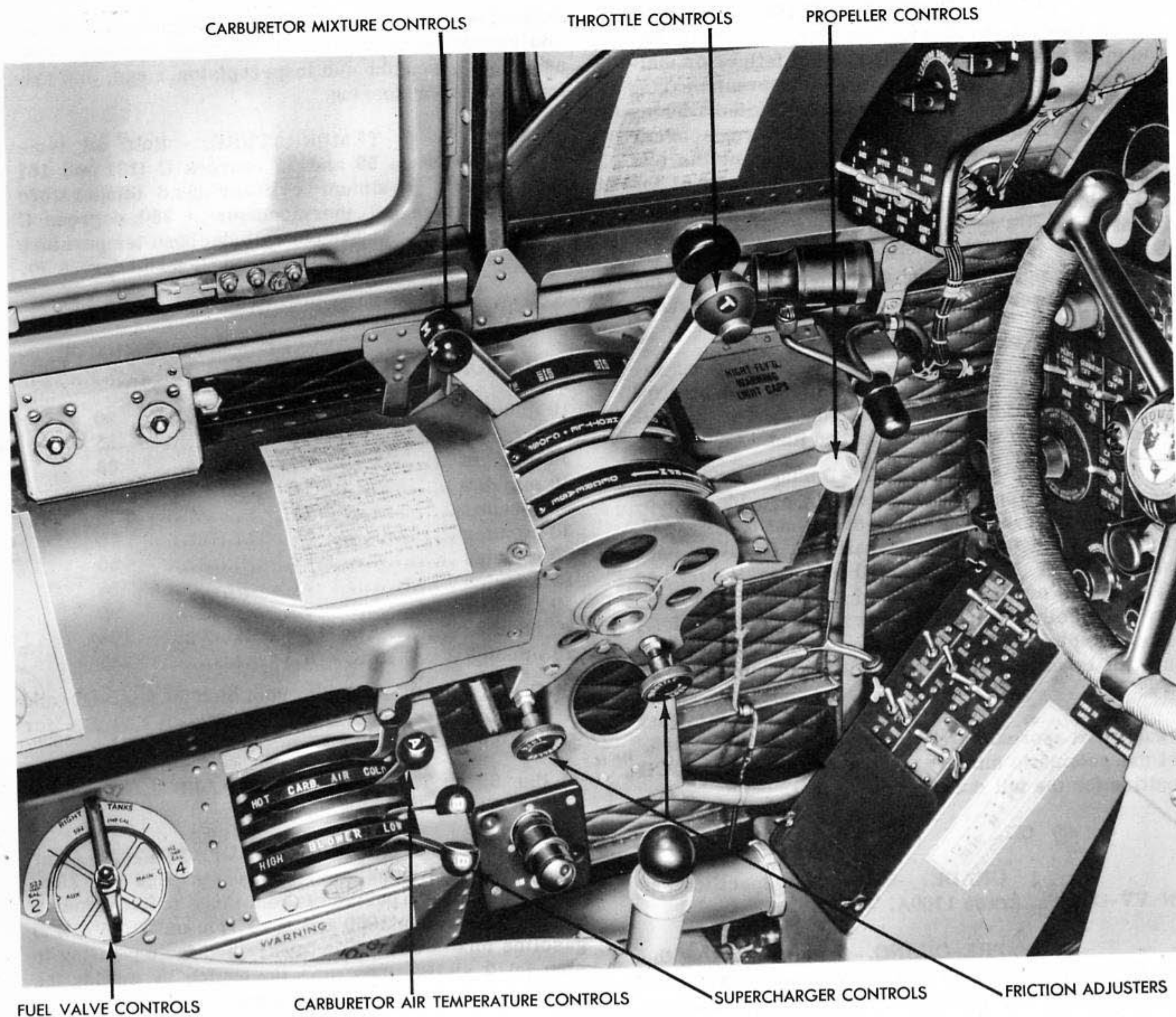
Figure 108 - INSTALLED ENGINE CONTROLS
