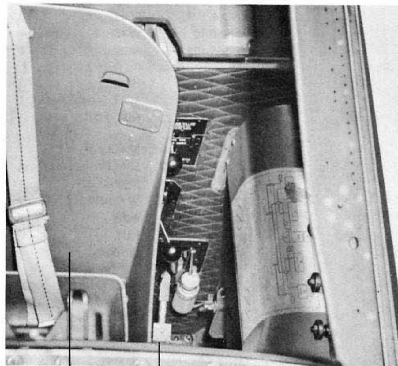
PILOT'S SEAT ALIGHTING GEAR HYDRAULIC CONTROL
