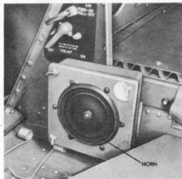
Figure 241 - ALIGHTING GEAR WARNING HORN
