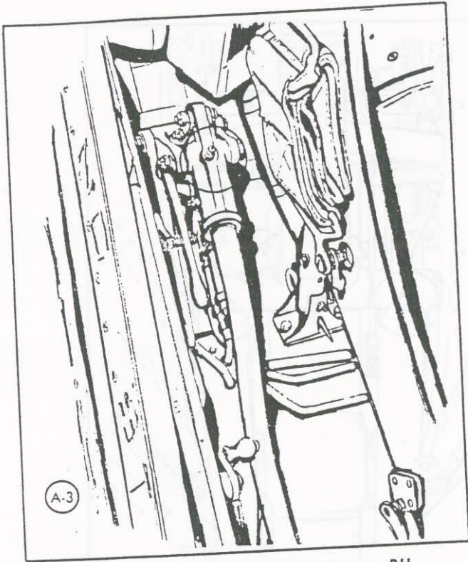
A-3 Emergency Hydraulic Hand Pump, RH Cockpit Floor
