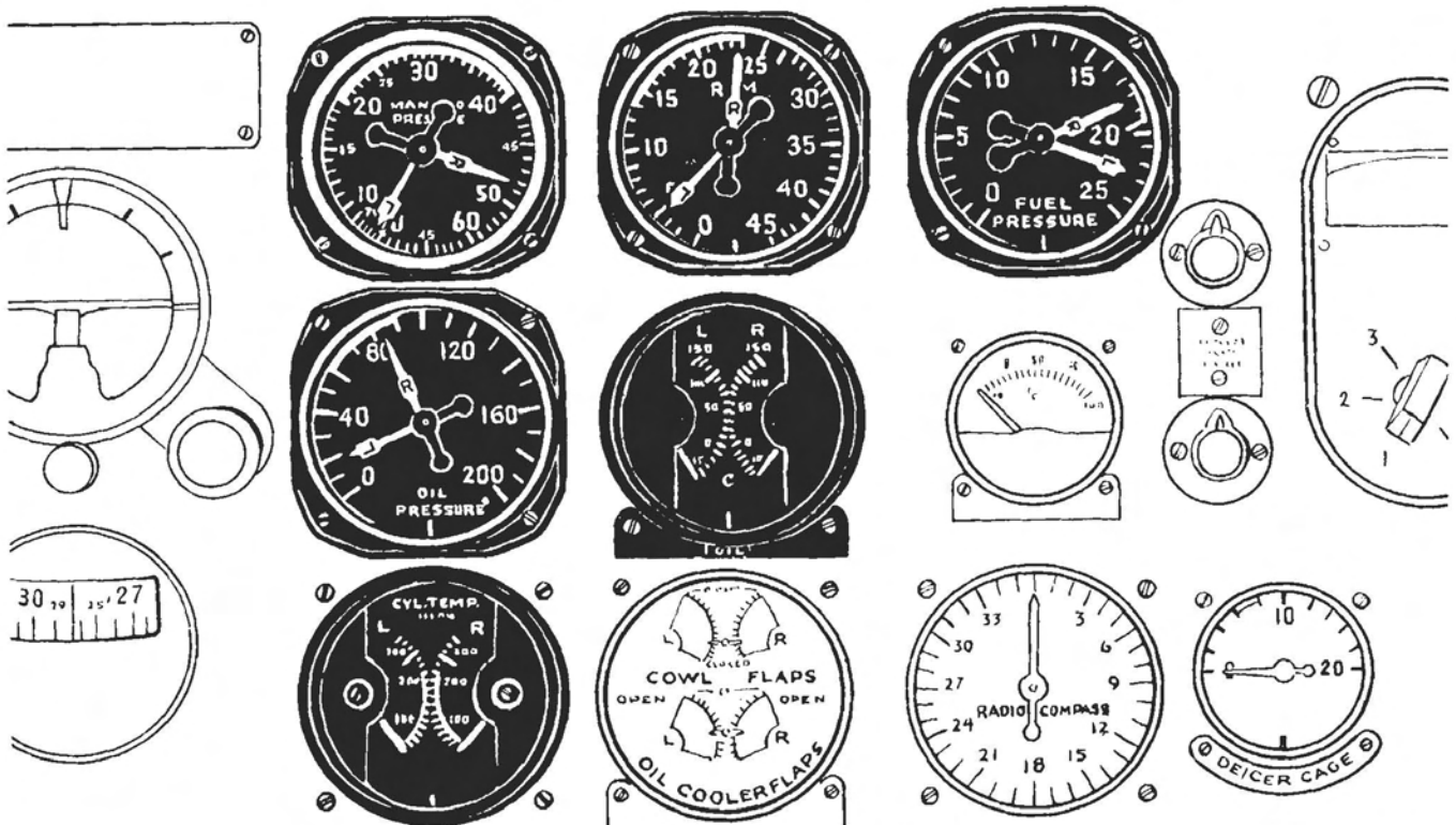
Figure 55—Temperature and Pressure Gages
