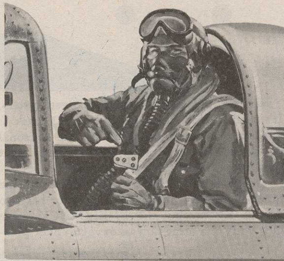
Clip oxygen hose to shoulder harness, not parachute harness, to afford quick getaway
