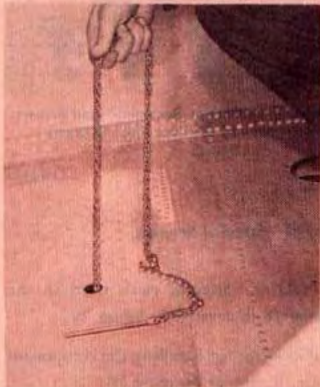
T6-FUEL TANK INSTALLATION CHAIN
