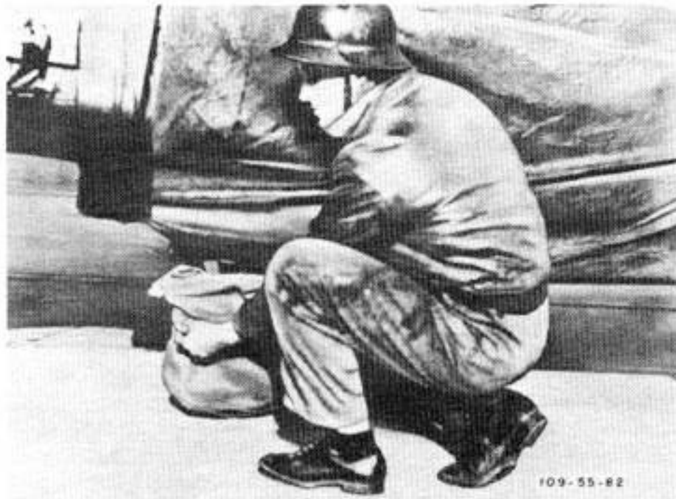
Figure 38—Installing Tail Wheel Cover
