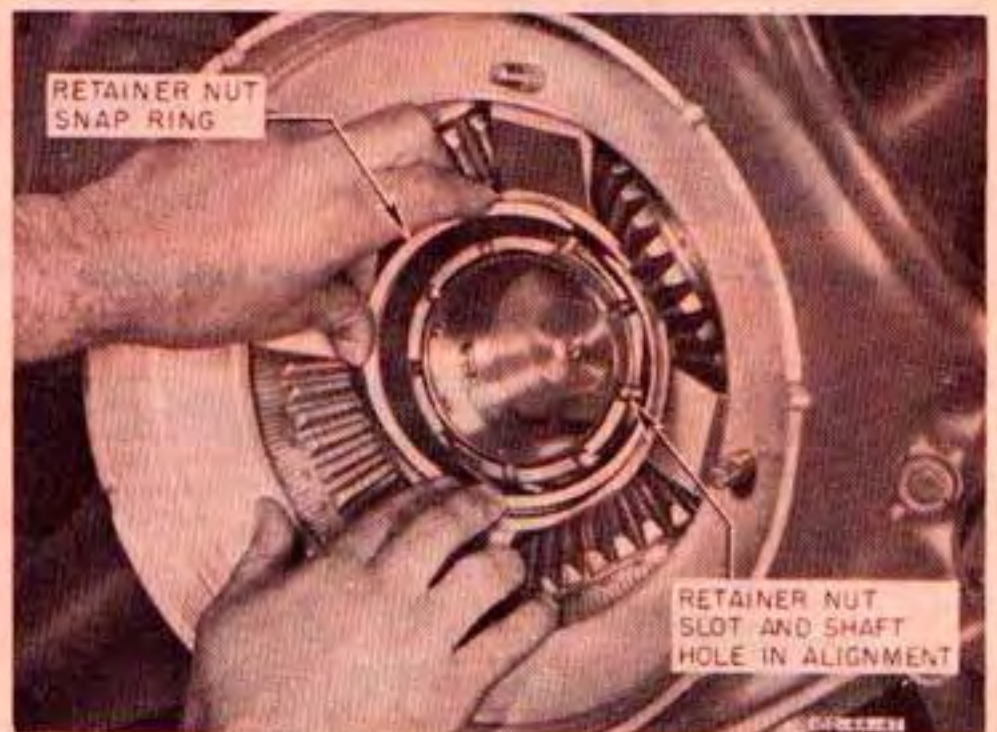
Figure 215—Installing Retainer Nut Snap Ring (Hamilton Standard)
