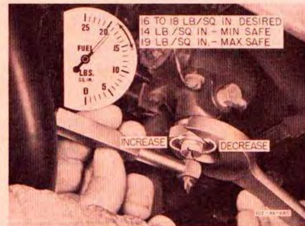
Figure 261—Adjusting Fuel Pressure
