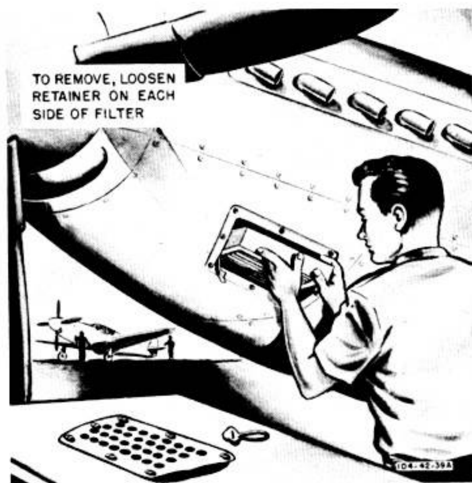
Figure 247—Removing Air Filters
