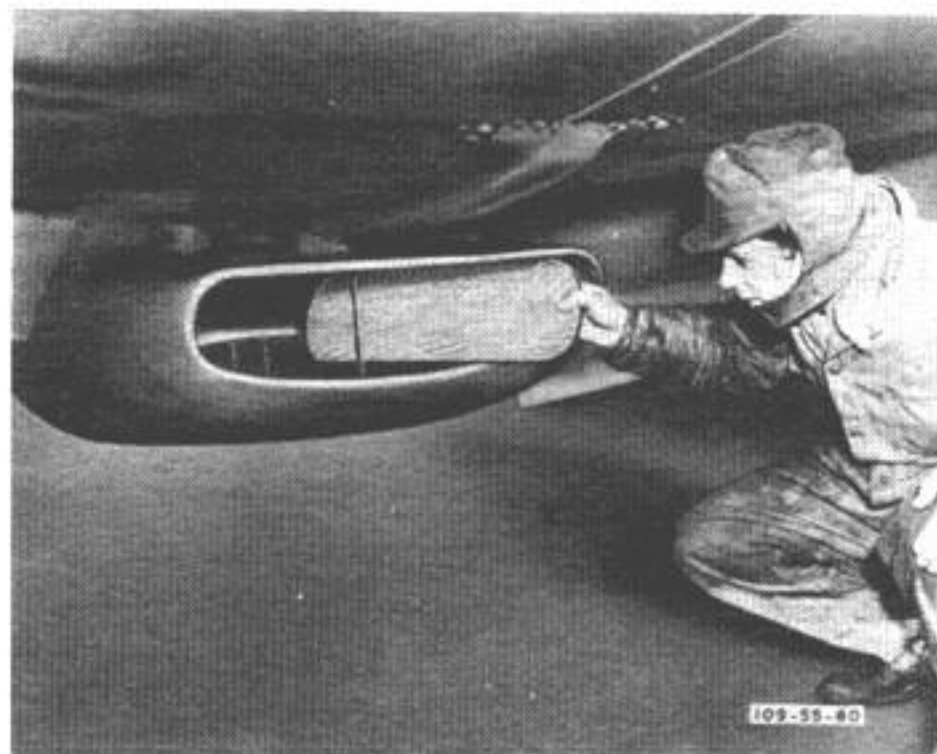
Figure 4—Placing Template Over the Oil Radiator Opening
