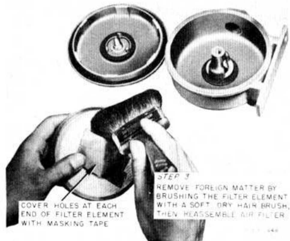
Figure 287—Cleaning Air Filter Elements (Purolator)
