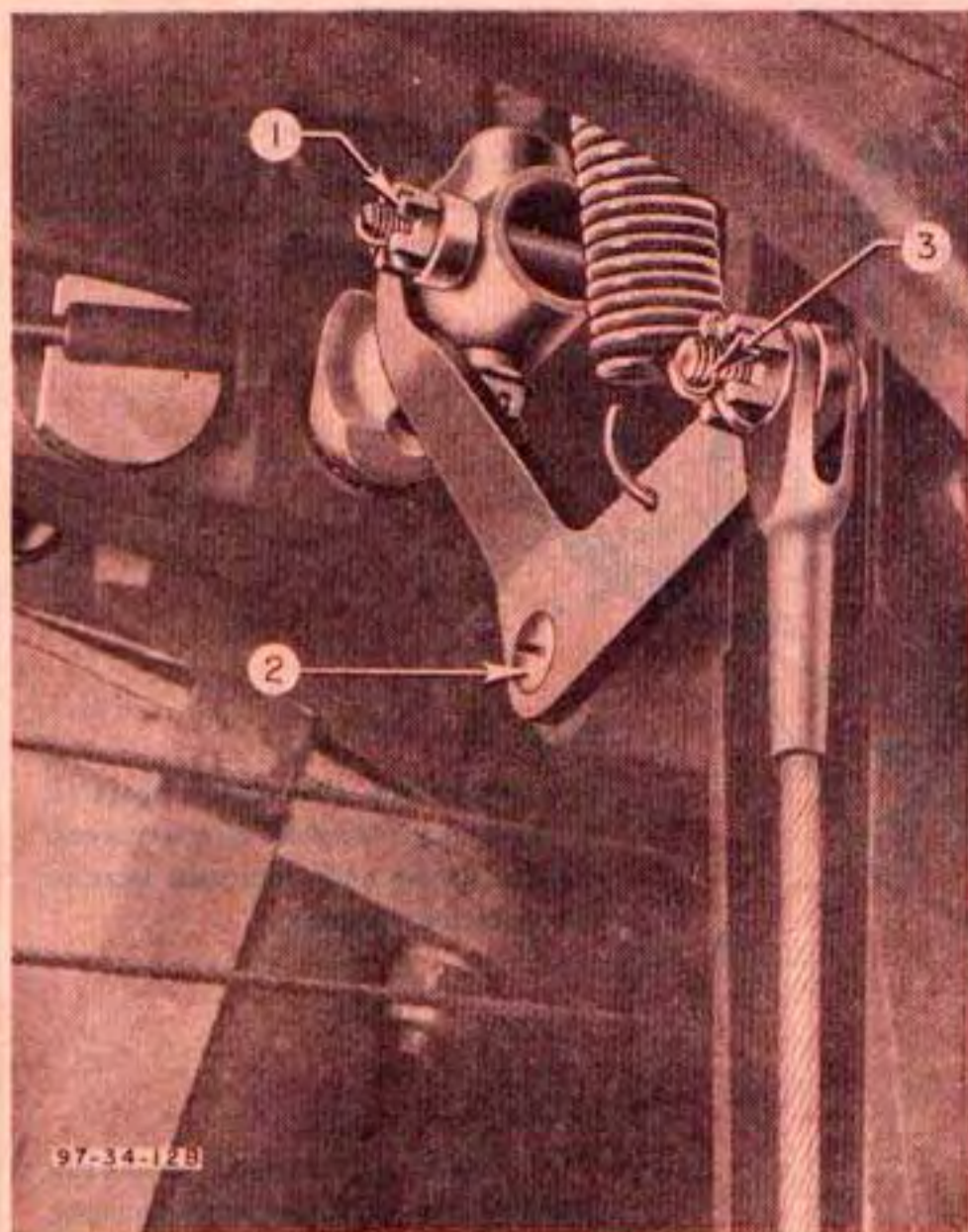
Figure 147—Tail Gear Down-lock
