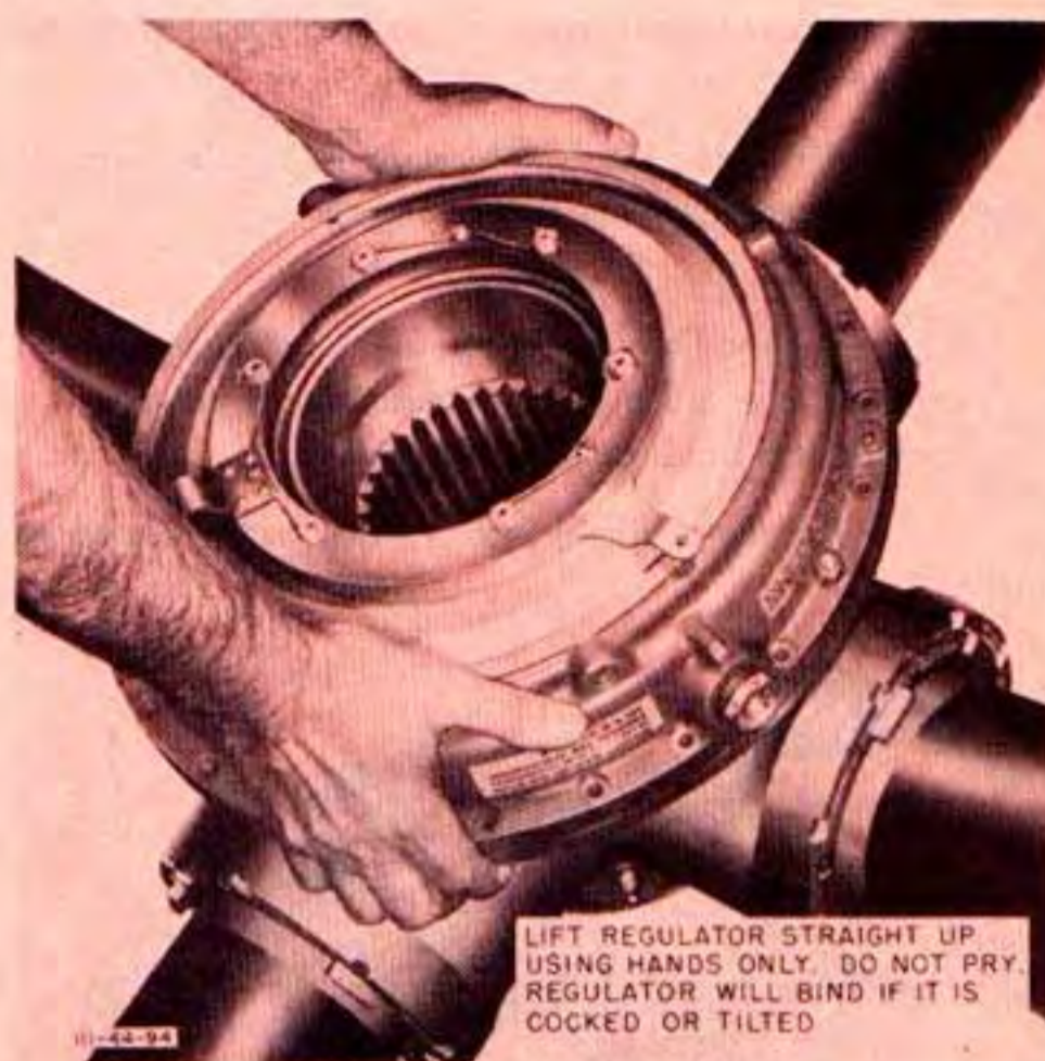
Figure 236J—Removing Regulator From Hub (Aeroproducts)
