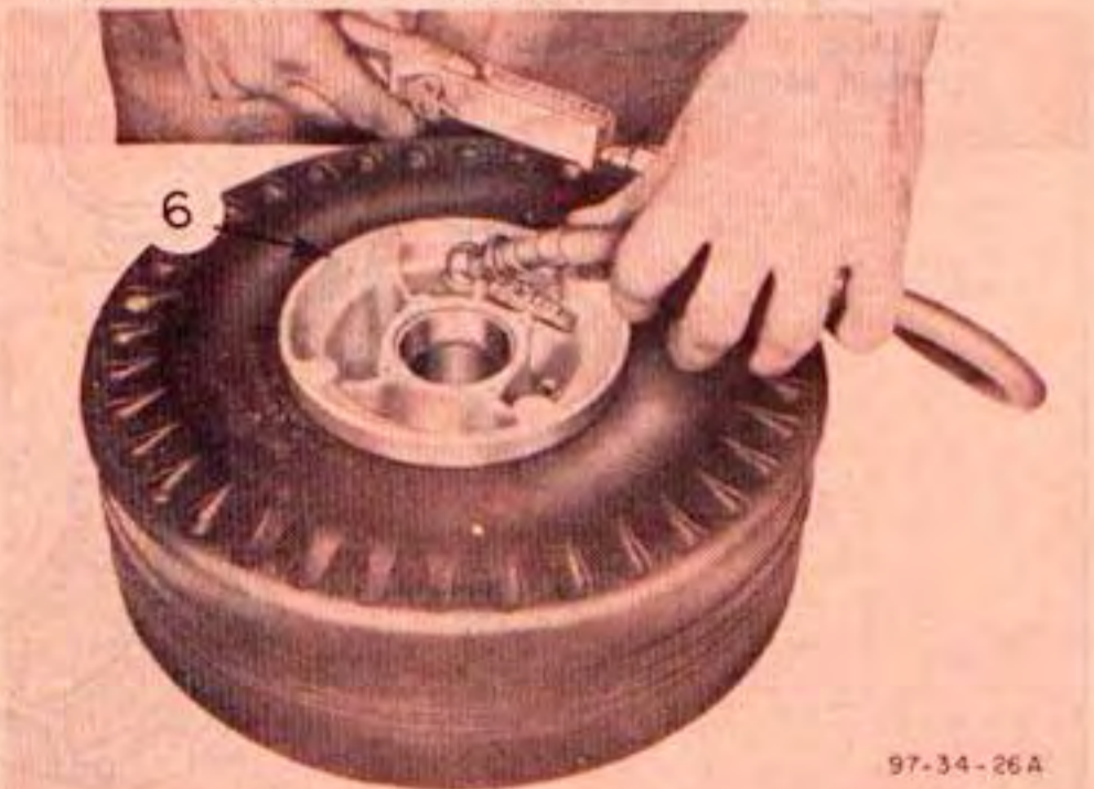
Figure 163—Mounting Tail Wheel Tire and Tube
