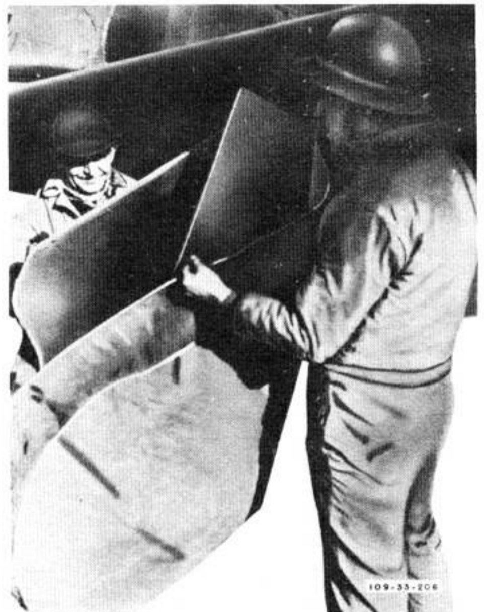
Figure 36—Installing Main Wheel Cover
