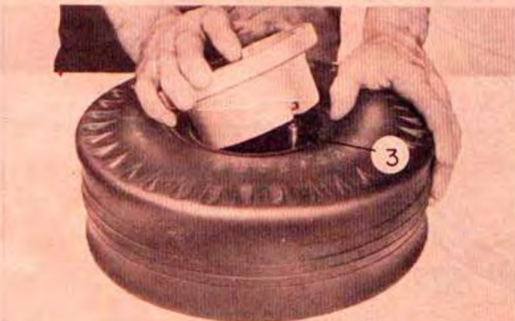
Figure 163—Mounting Tail Wheel Tire and Tube
