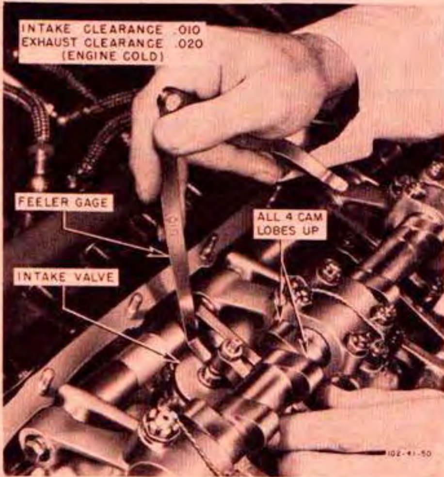
Figure 168—Checking Valve Clearances
