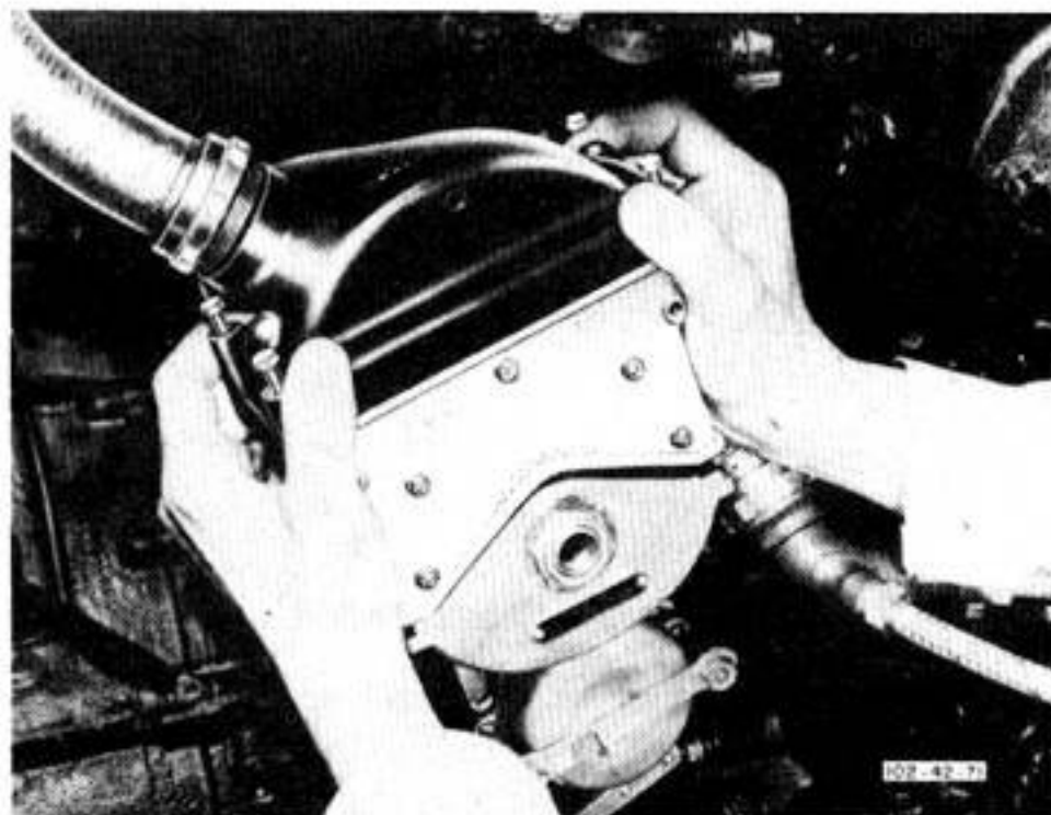
Figure 181—Removing Harness and Distributor Covers
