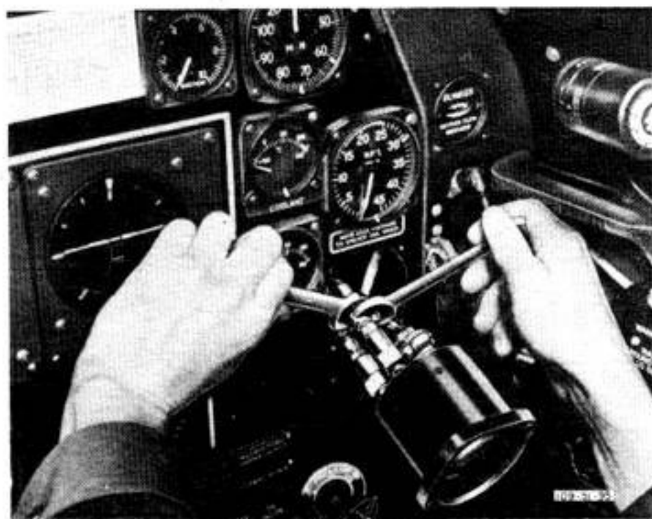
Figure 278—Removing Front Mounted Instrument
