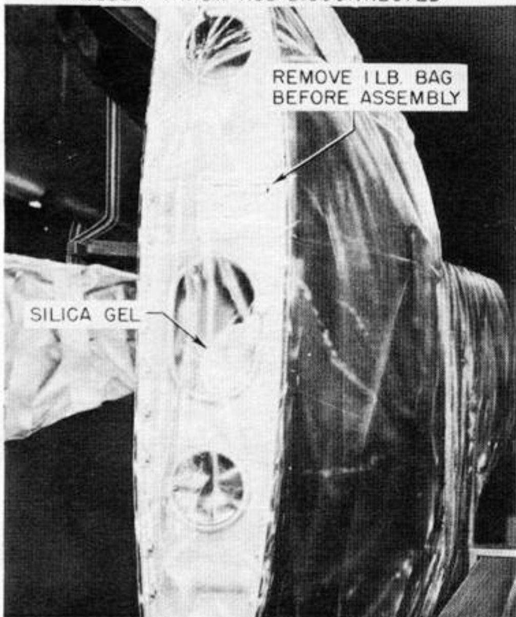
SILICA GEL BAGS INSTALLED
