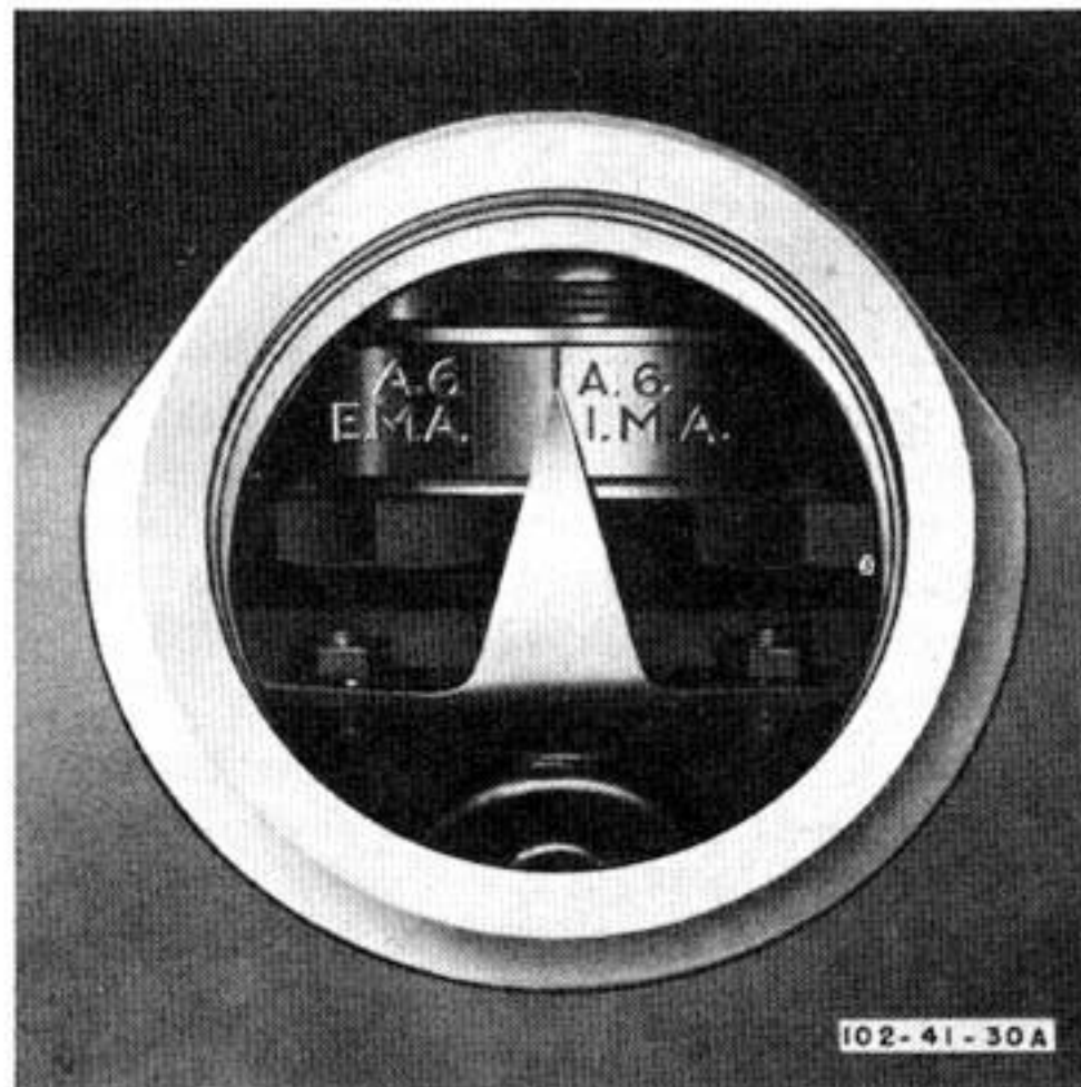
Figure 183—Crankshaft Magneto Timing Position
