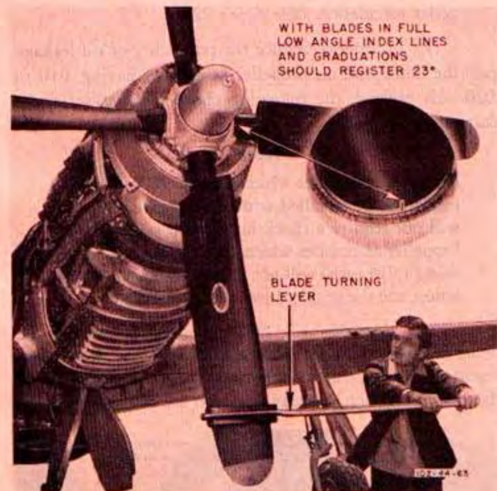
Figure 233—Turning Blades to Low Pitch (Hamilton Standard)
