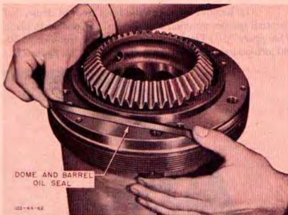
Figure 227—Installing Dome Oil Seal (Hamilton Standard)
