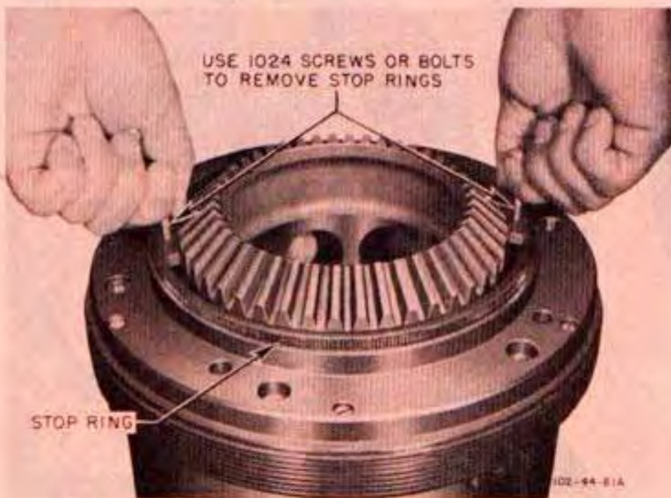
Figure 221—Removing Stop Rings (Hamilton Standard)
