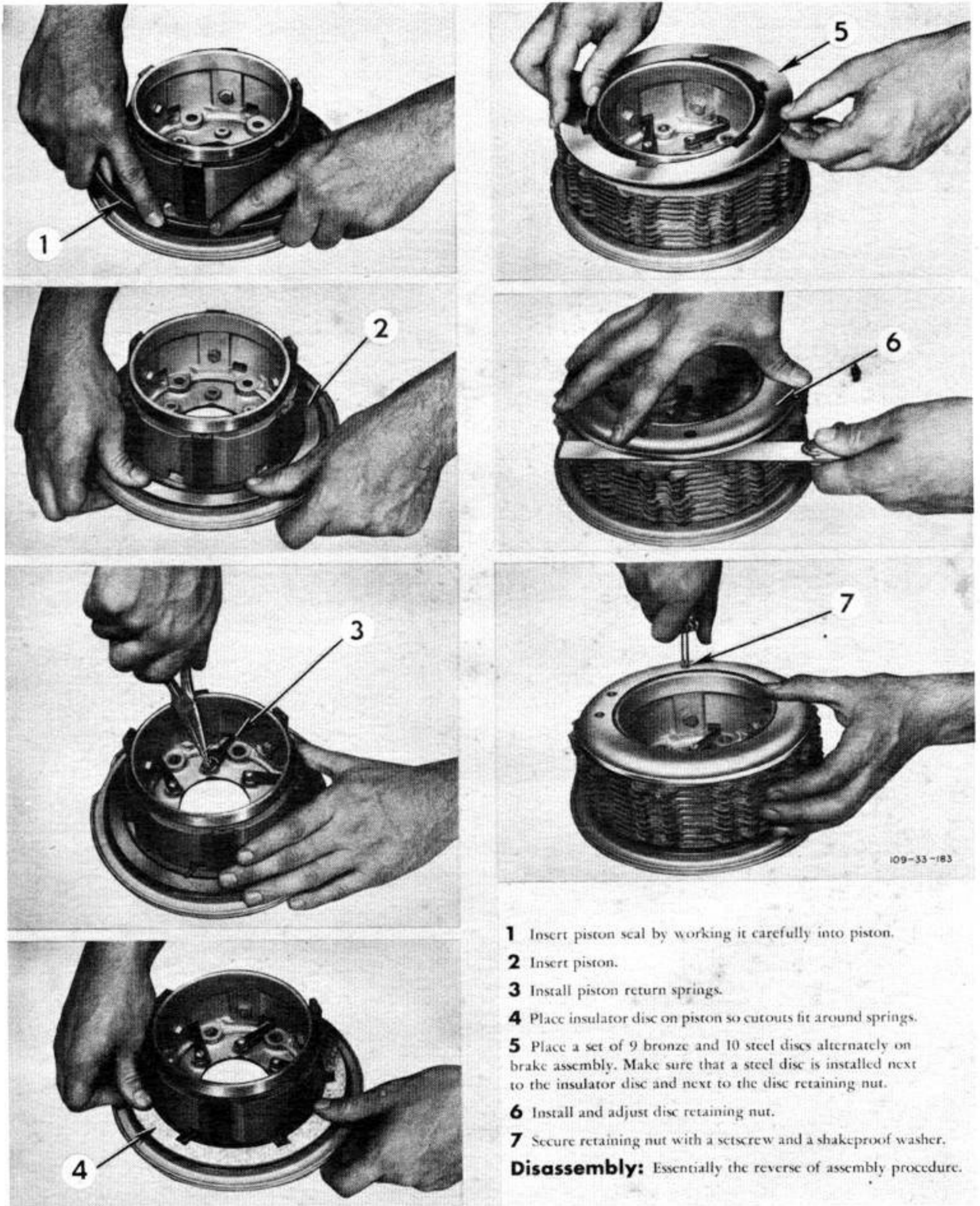
Figure 155—Assembling Disc Brake
