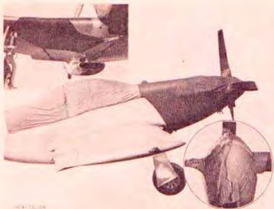
Figure 459—Weatherproof Covers Installed
