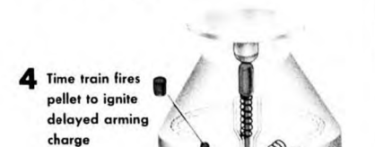
3 Delay firing pin springs up to hit primer which fires time train
