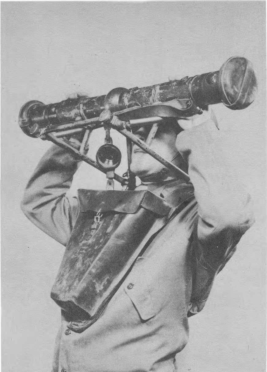
FIGURE 22. - POSITION OF EM 34 WITH CARL ZEISS SHOULDER HARNESS WHEN SIGHTING AIRCRAFT TARGET
