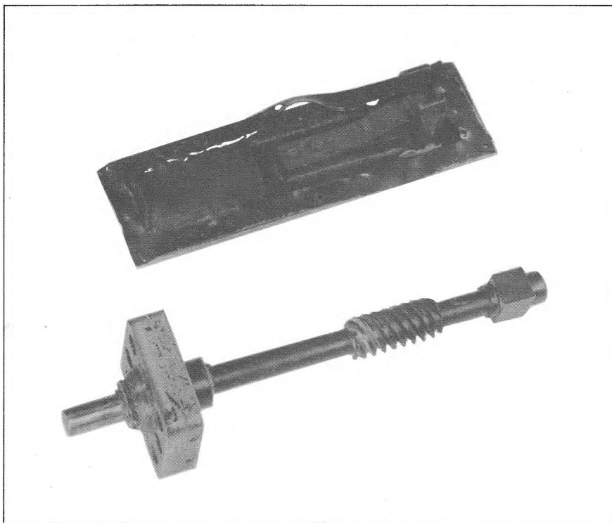
FIGURE 79. - JAPANESE HEIGHT FINDER, 2-METER BASE - ELEVATION WORM AND ANTI-BACKLASH SPRING ASSEMBLY
