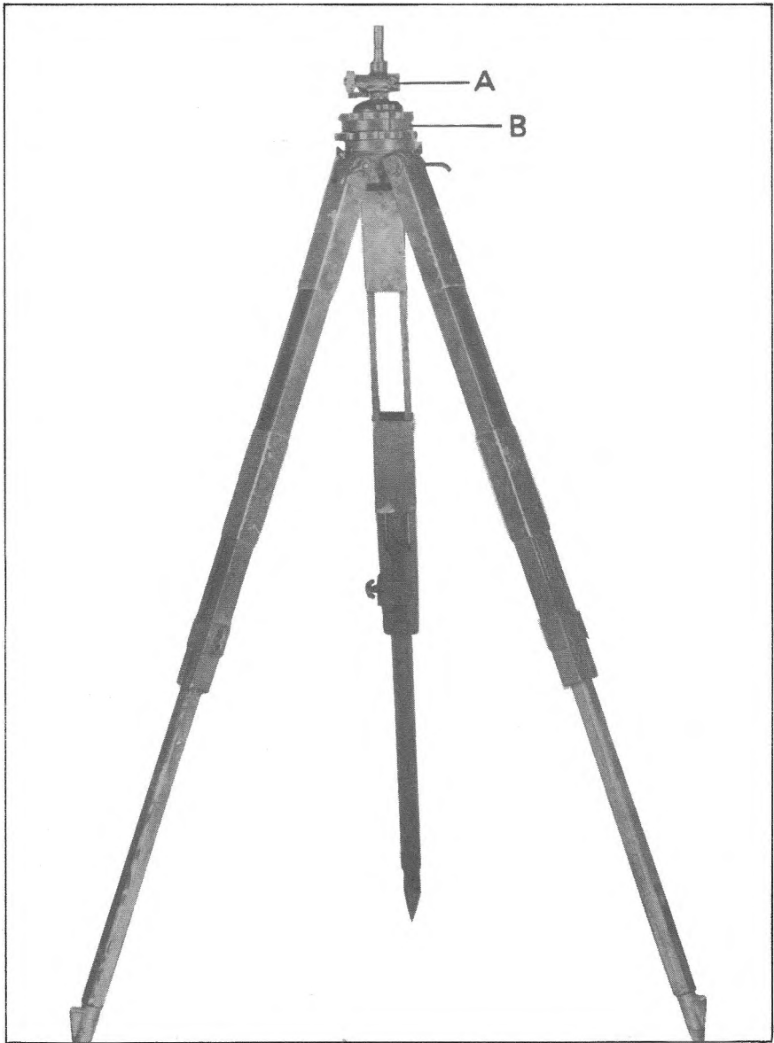
FIGURE 13. - TRIPOD AND MOUNTS FOR TELESCOPE, B.C.
