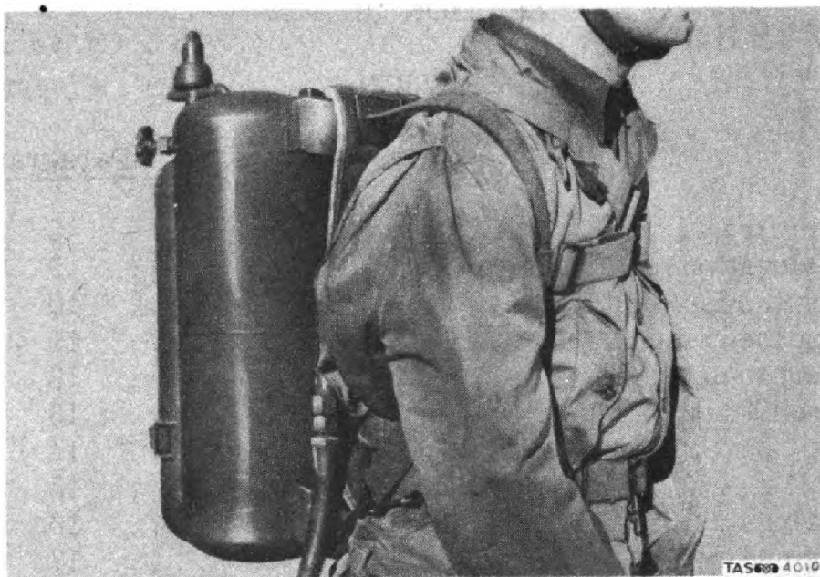
Figure 12. Correct Method of Carrying Fuel Unit, With Weight Distributed on the Straps.
