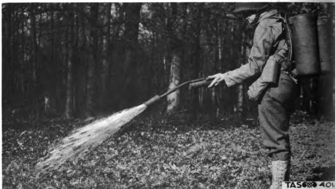
Figure 19. After Firing and Returning to a Safe Position, Remaining Fuel Is Blown from Gun Toward Ground.
