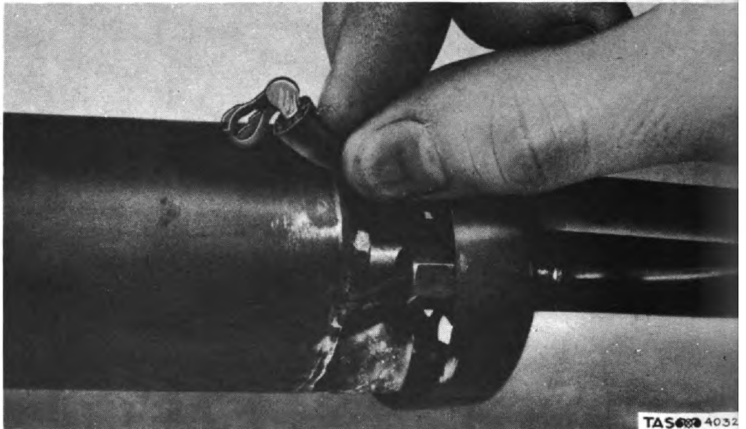
Figure 42. Touching Spark Plug Lead Wire Clip to Gun to Test for Spark.
