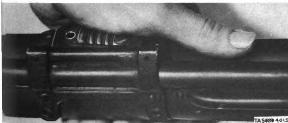
Figure 17. Trigger Safety Key Forced Down and Forward With Heel of Thumb, Actuating Electrical and Hydrogen Systems.
