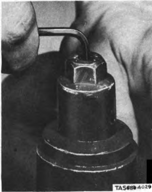
Figure 39. Adjusting Pressure Regulator, Using Hollow Set-Screw Hexagonal Wrench on the Adjusting Screw. Seal Has Been Removed.
