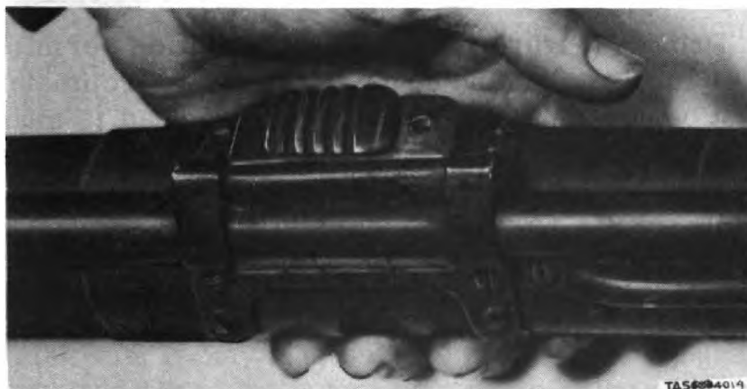
Figure 16. Trigger Safety Key in Safe Position, Before Heel of Thumb Vigorously Strikes and Slides It Forward.
