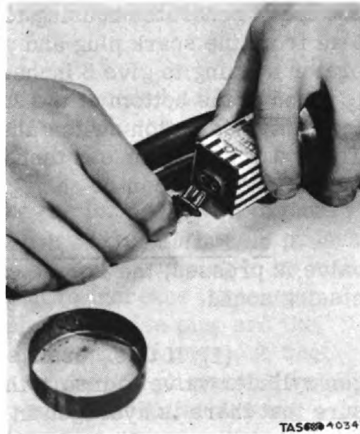
Figure 44. Battery Removed from Spark Generator Housing with Plug Pulled from Battery. Housing Cap Is in Foreground.
