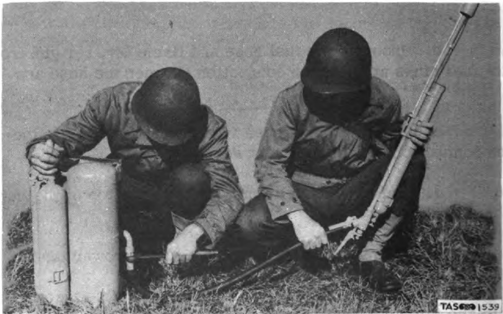
Figure 28. Attaching Gun to Filled Flame Thrower.
