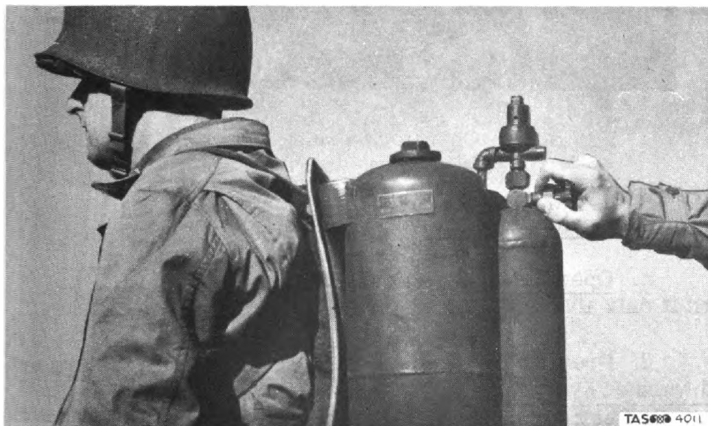
Figure 13. Assistant Opening the Pressure Cylinder Valve Before Operator Is in Position to Fire.
