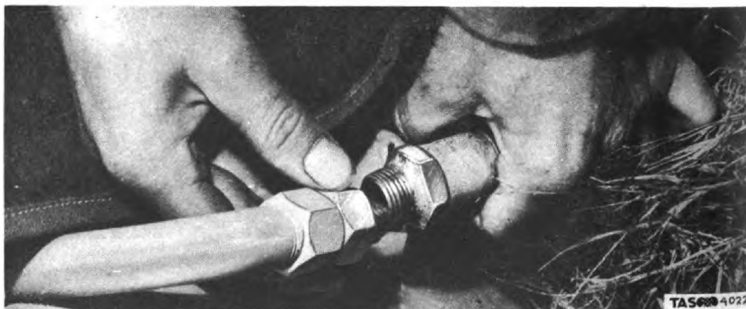
Figure 22. Uncoupling Hose from Hose Connector.
