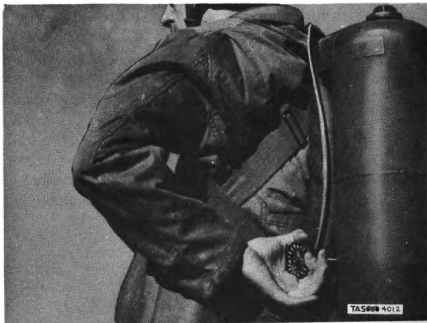
Figure 14. Operator Opening the Fuel Valve Preparatory to Firing.
