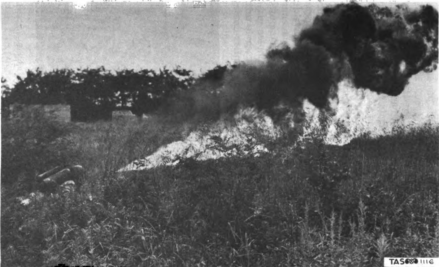
Figure 24. Firing with Liquid Fuel. Range Is Shorter and Fuel Is Largely Burned in Flight. Screening Effect Is Useful.
