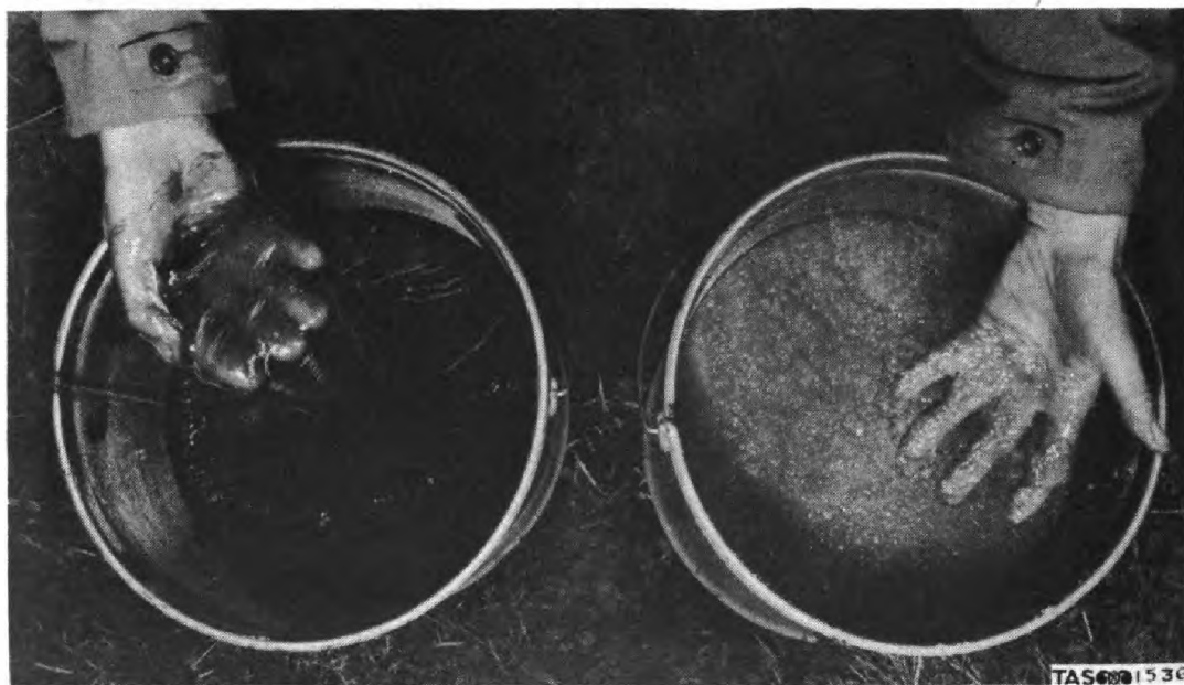
Figure 25. Contrasting Newly Mixed Thickened Fuel (Right) with "Aged" Fuel (Left).
