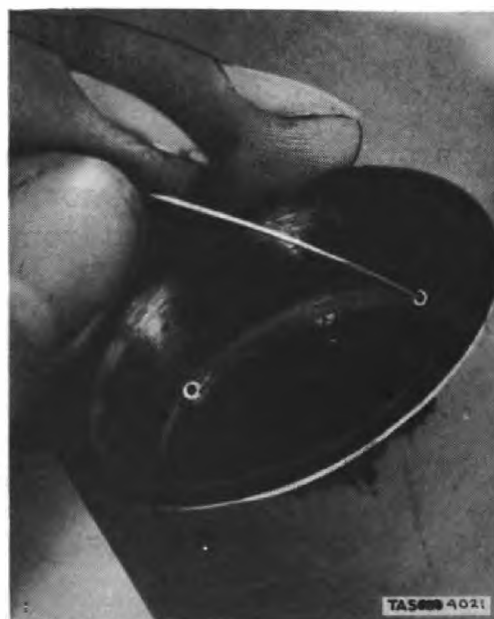
Figure 21. Cleaning Each of 20 Orifices of Gas Burner with Sliver of Wood or Iron Wire After Firing.
