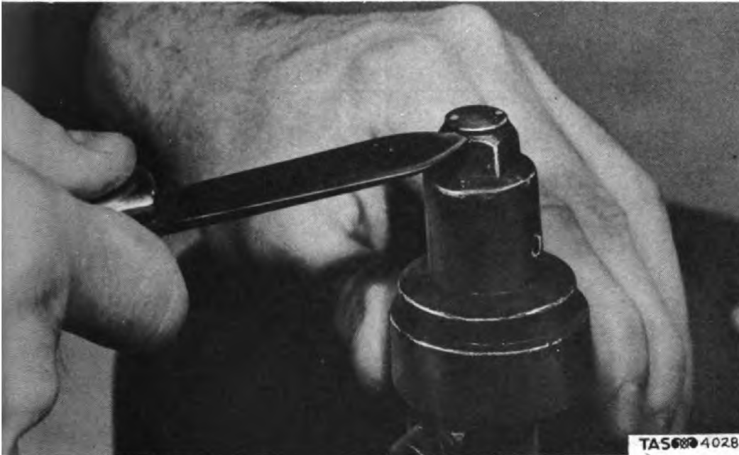
Figure 38. Unprying Adjusting Screw Seal and Two Drive Screws on Pressure Regulator by Using Knife Blade.
