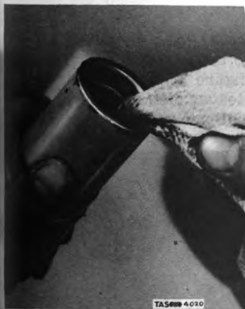
Figure 20. Cleaning Gas Burner With Cloth After Firing. Entire Inside Must Be Wiped.
