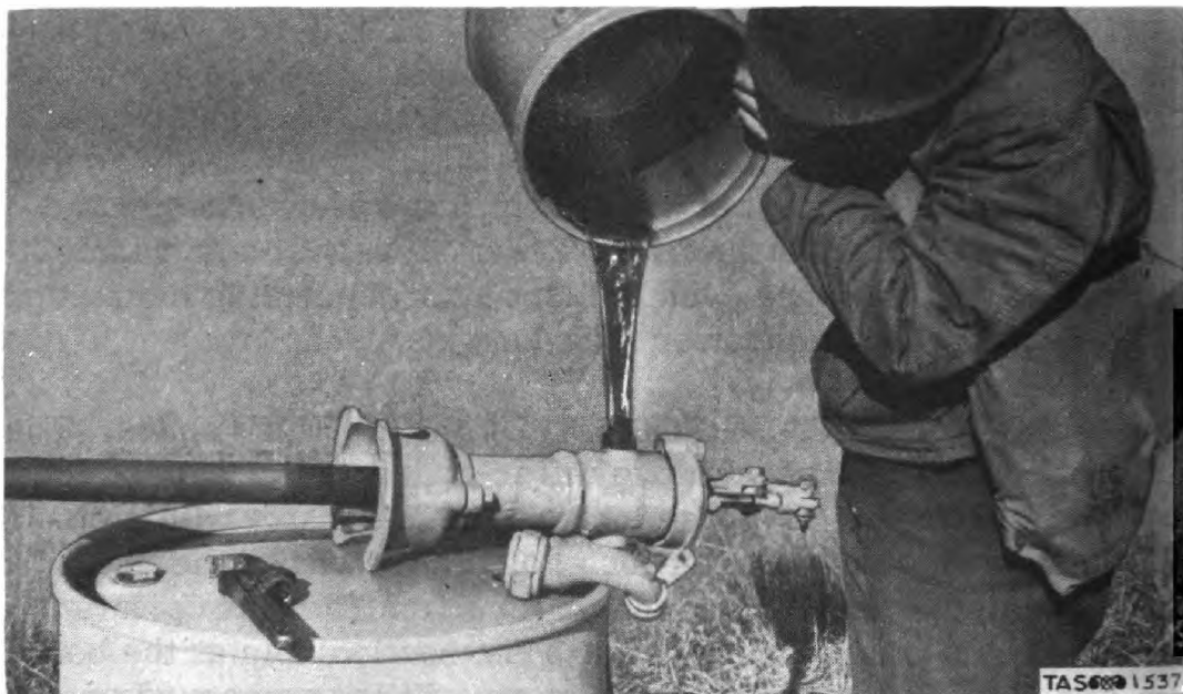
Figure 26. Priming the Pump.
