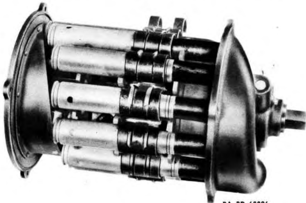
Figure 48 — Separation of Links from Rounds in 20-MM Feed Mechanism AN-M1 — Right Side View
