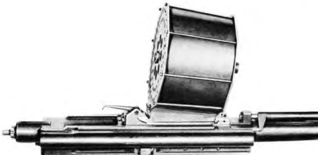
Figure 67 – Loaded Magazine in Position on Gun
