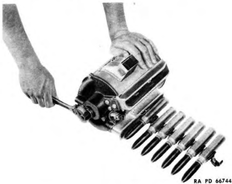
Figure 57 — Loading R.H. Feed Mechanism
