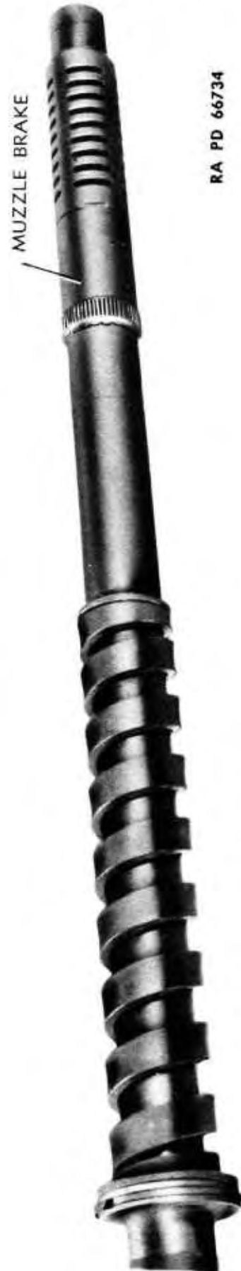
Figure 32 — 20-MM Adapter M7 with Muzzle Brake
