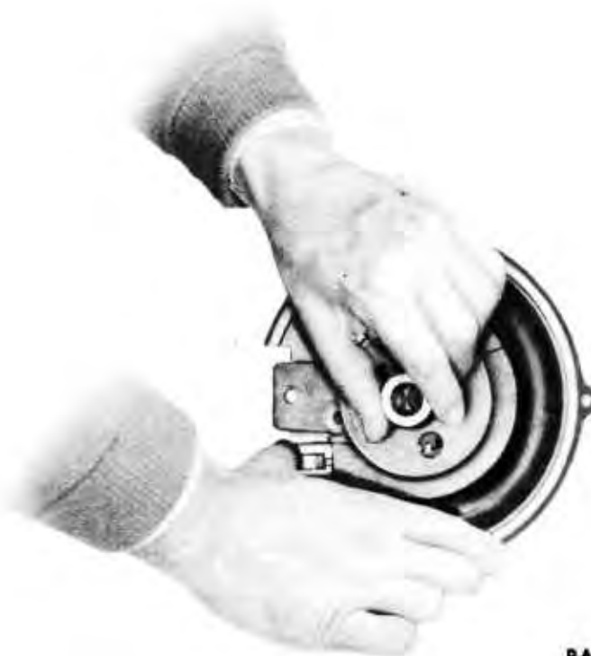
Figure 89 – Engaging Rack to Ratchet Segment
