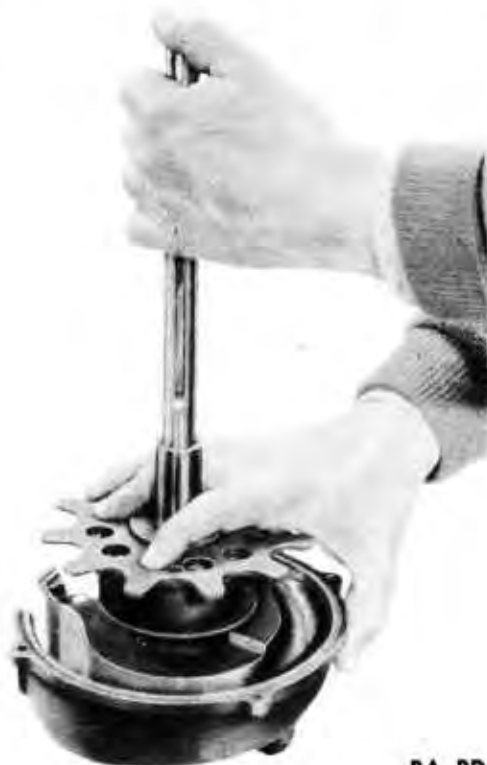
Figure 90 – Inserting Shaft into Hub
