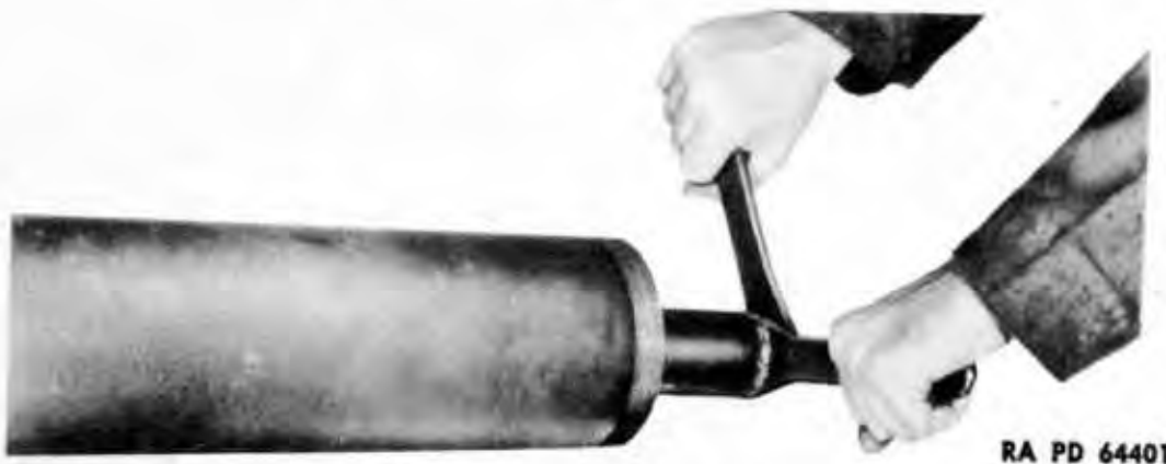
Figure 127 – Tightening Lock Nut Against Adjusting Nut
