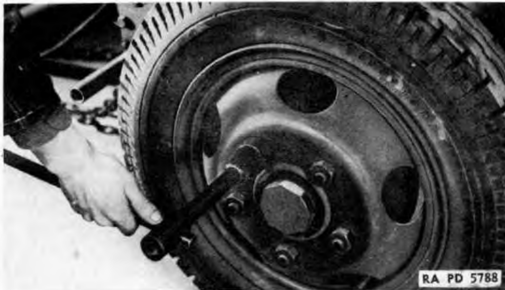
Figure 140 — Removal of Wheel
