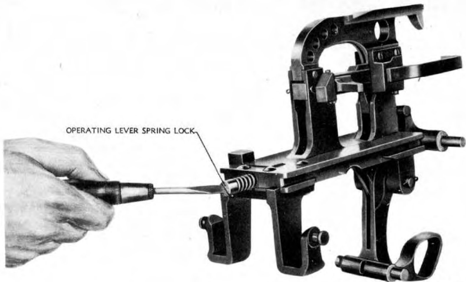
Figure 74 — Removing Operating Lever Spring Lock Assembly
