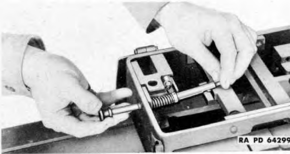
Figure 115 — Removing Cartridge Feeder Pawl Handle, Spring, and Connector Shaft
