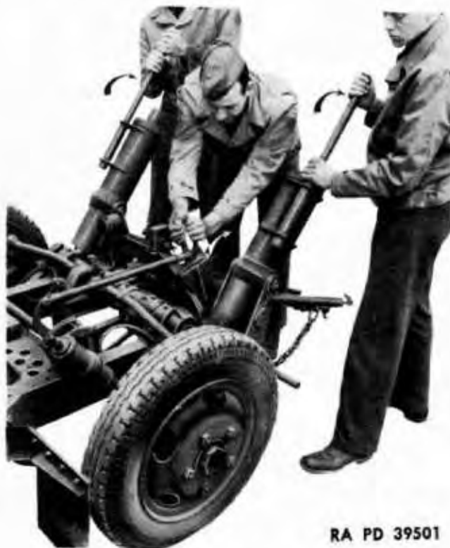
Figure 39 — Lowering Front of Carriage to Firing Position
