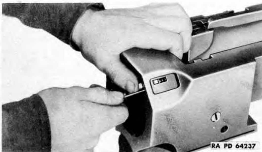
Figure 96 — Releasing Tube Lock Plate Plunger
