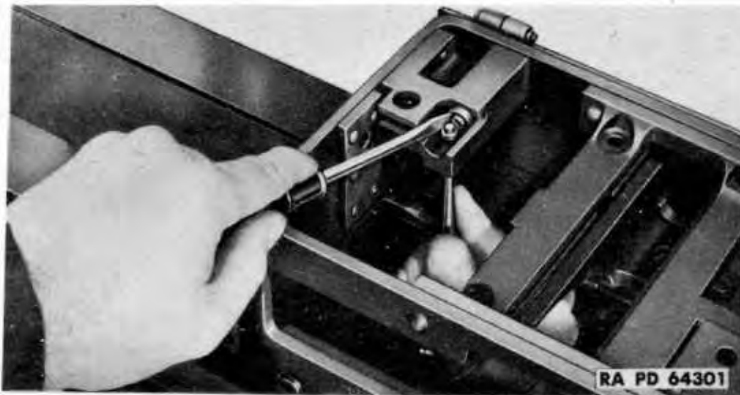
Figure 117 – Removing Feed Slide Return Lever Plunger and Spring
