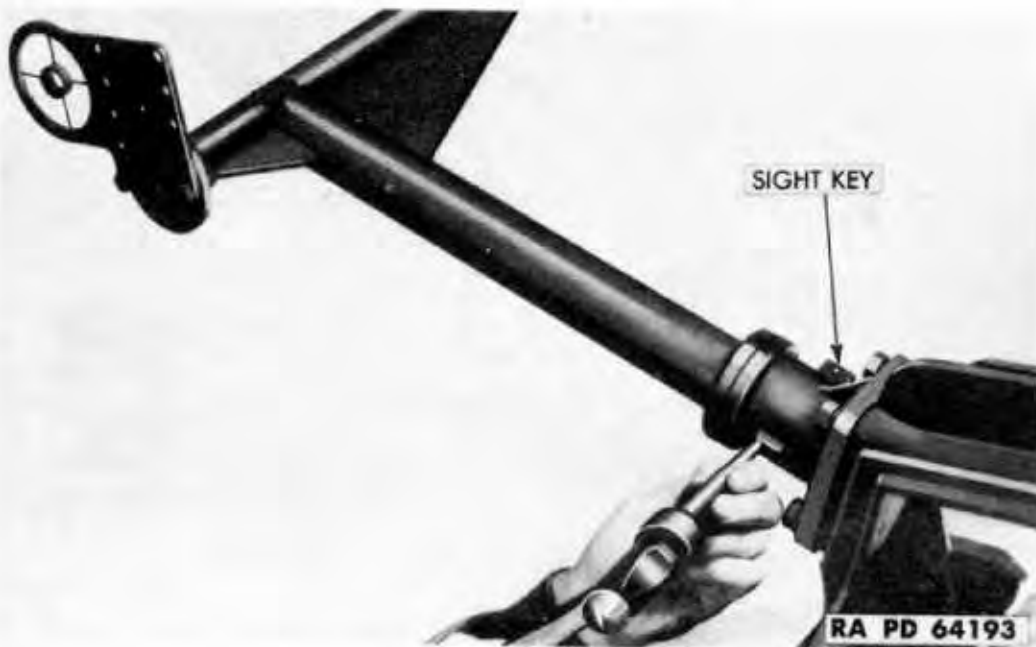
Figure 125 — Removing Sight Key
