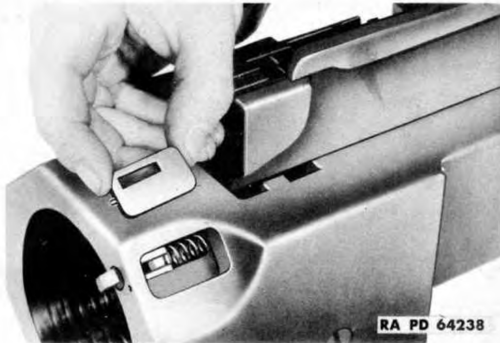
Figure 97 — Removing Tube Lock Plate Assembly
