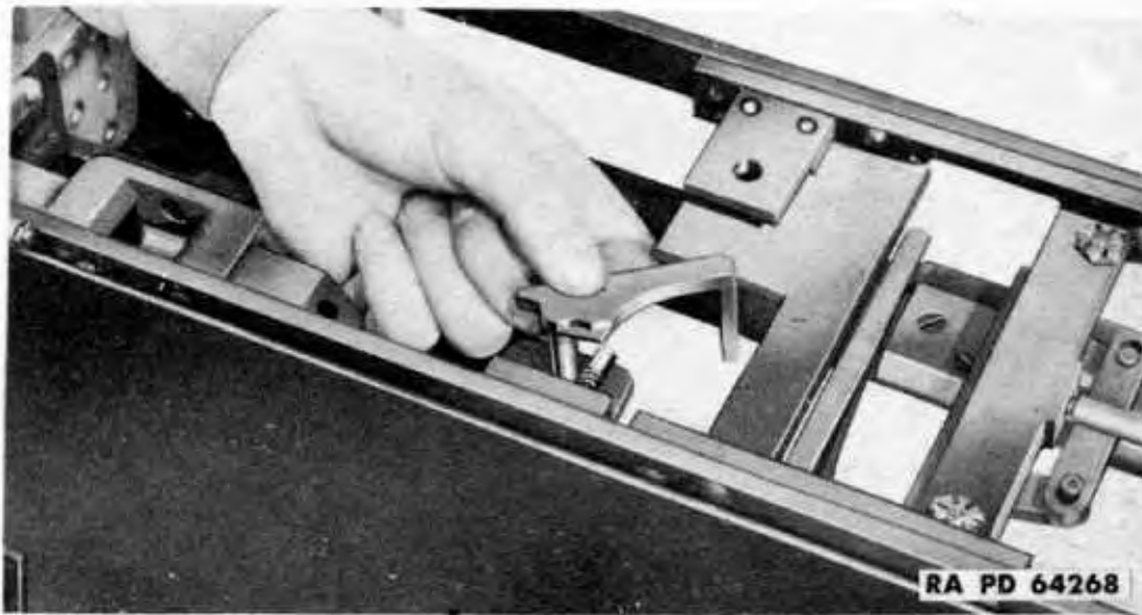
Figure 113 — Removing Carrier Catch
