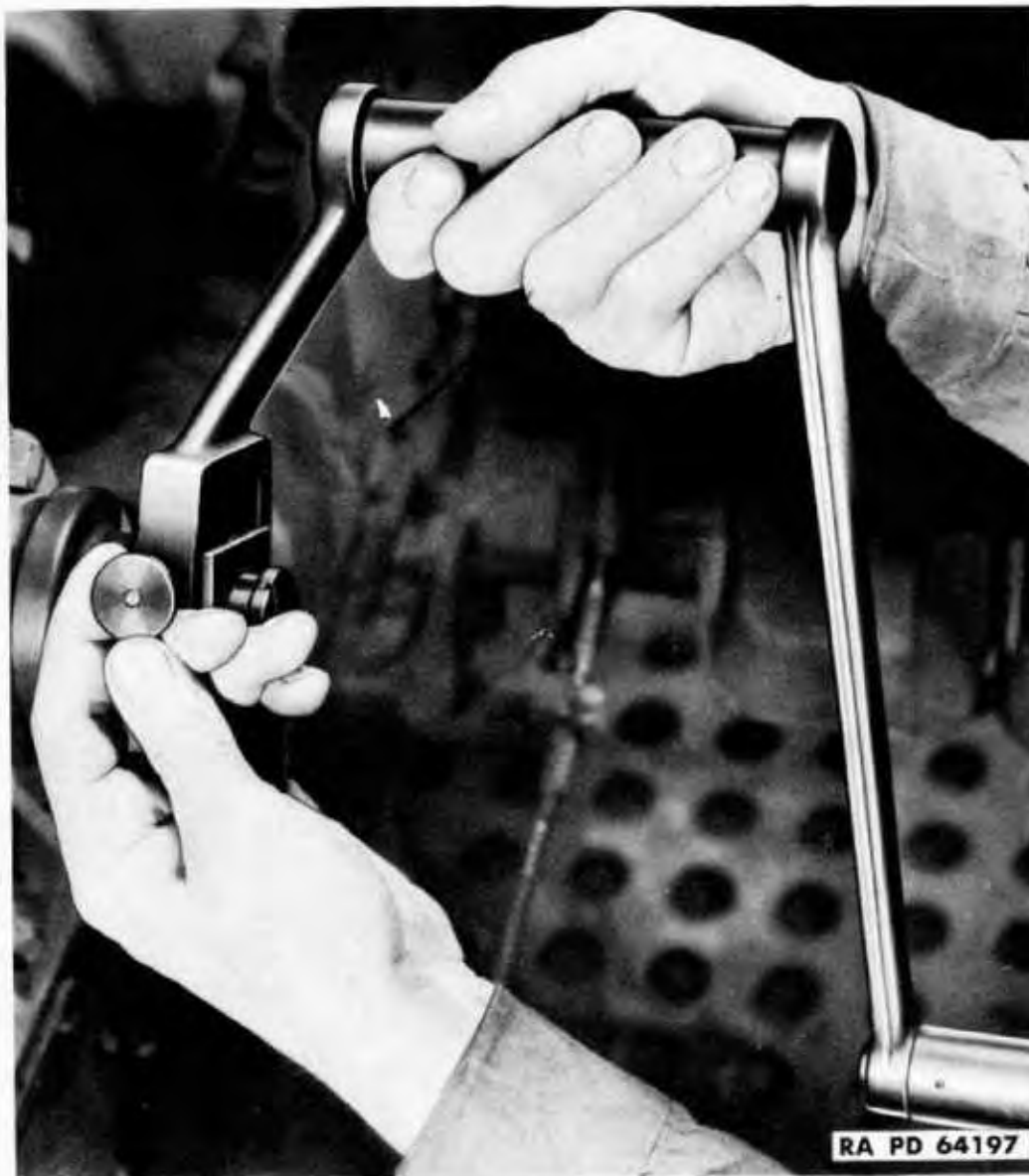
Figure 49 — Removing Hand Crank
