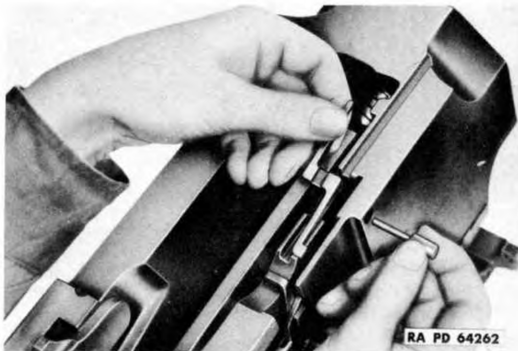
Figure 98 — Removing Trigger Trip
