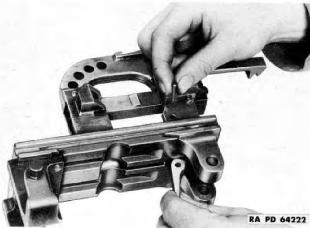
Figure 77 — Removing Cocking Lever
