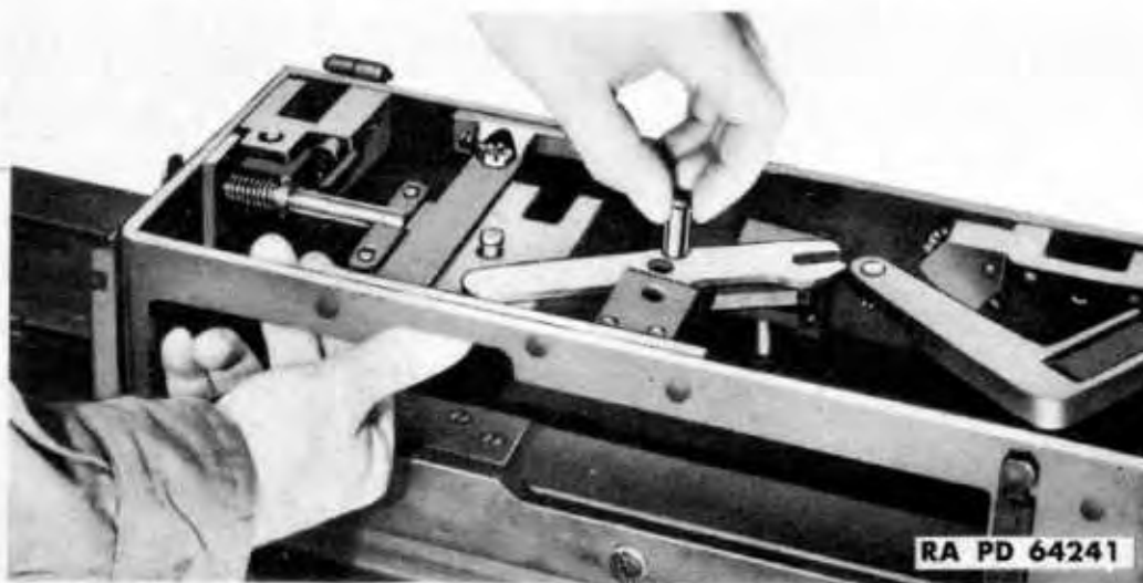
Figure 108 — Removing Feed Slide Lever
