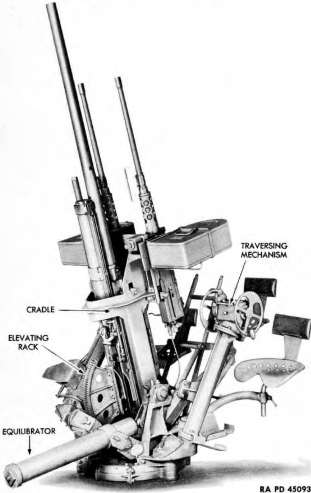
Figure 38 — Combination Gun Mount M42 — Guns Elevated 85 Degrees
