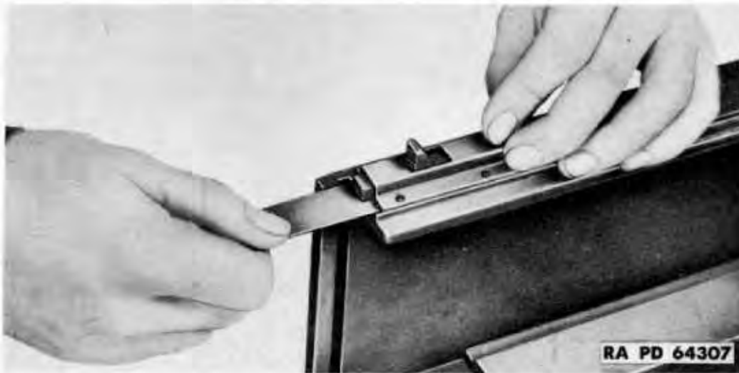
Figure 123 – Installing Back Plate Latch Assembly
