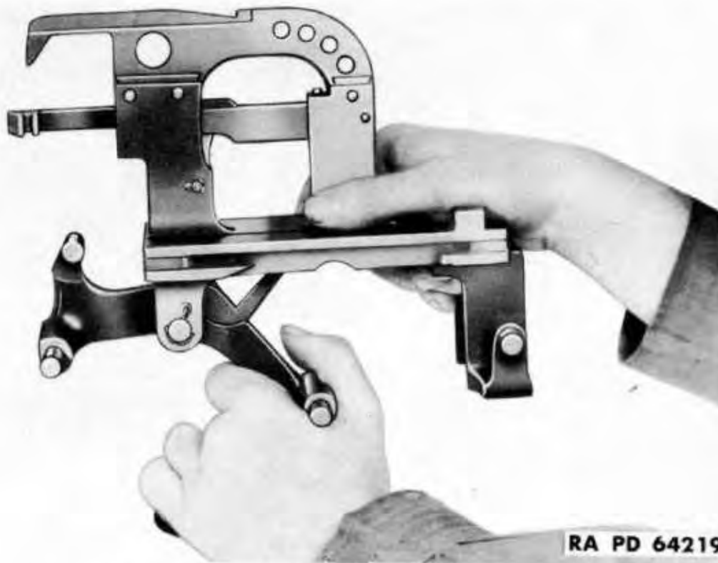
Figure 73 – Easing Operating Lever Forward
