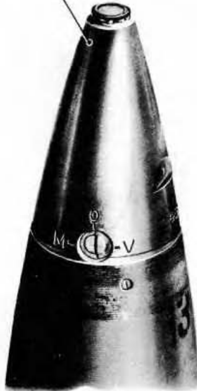
Figure 74 — Spring-wound Time, Percussion, and Inertia-operated Time Fuzes for German 88-mm High-explosive Shell — View Showing Setter Grooves and Selector Element
