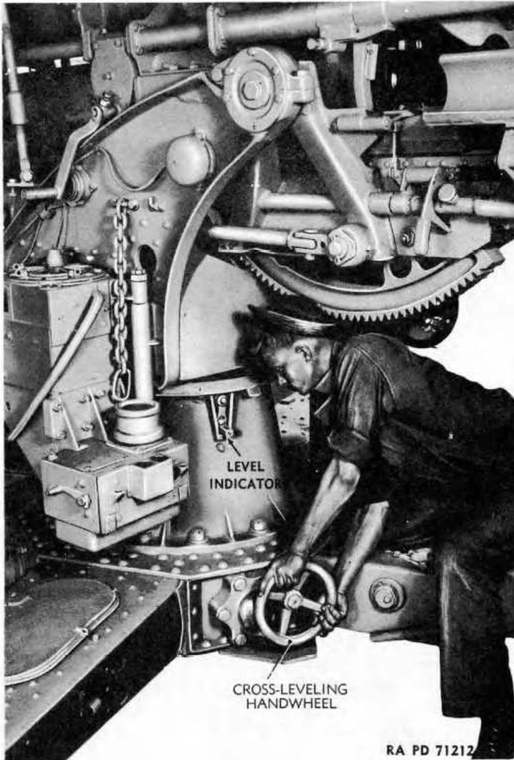
Figure 39 — Leveling Top Carriage
