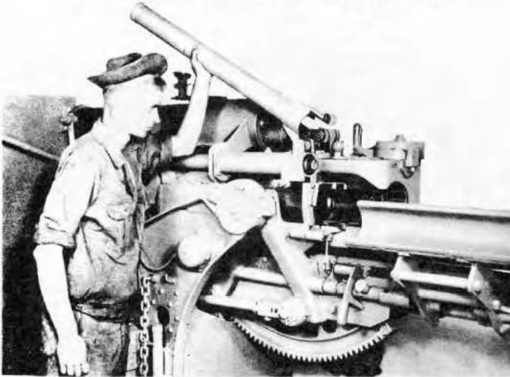
Figure 40 — Unfolding Rammer Guard
