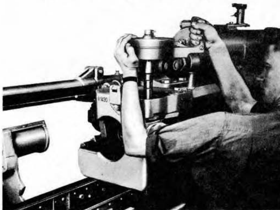
Figure 63 — Removing Breech Actuating Mechanism
