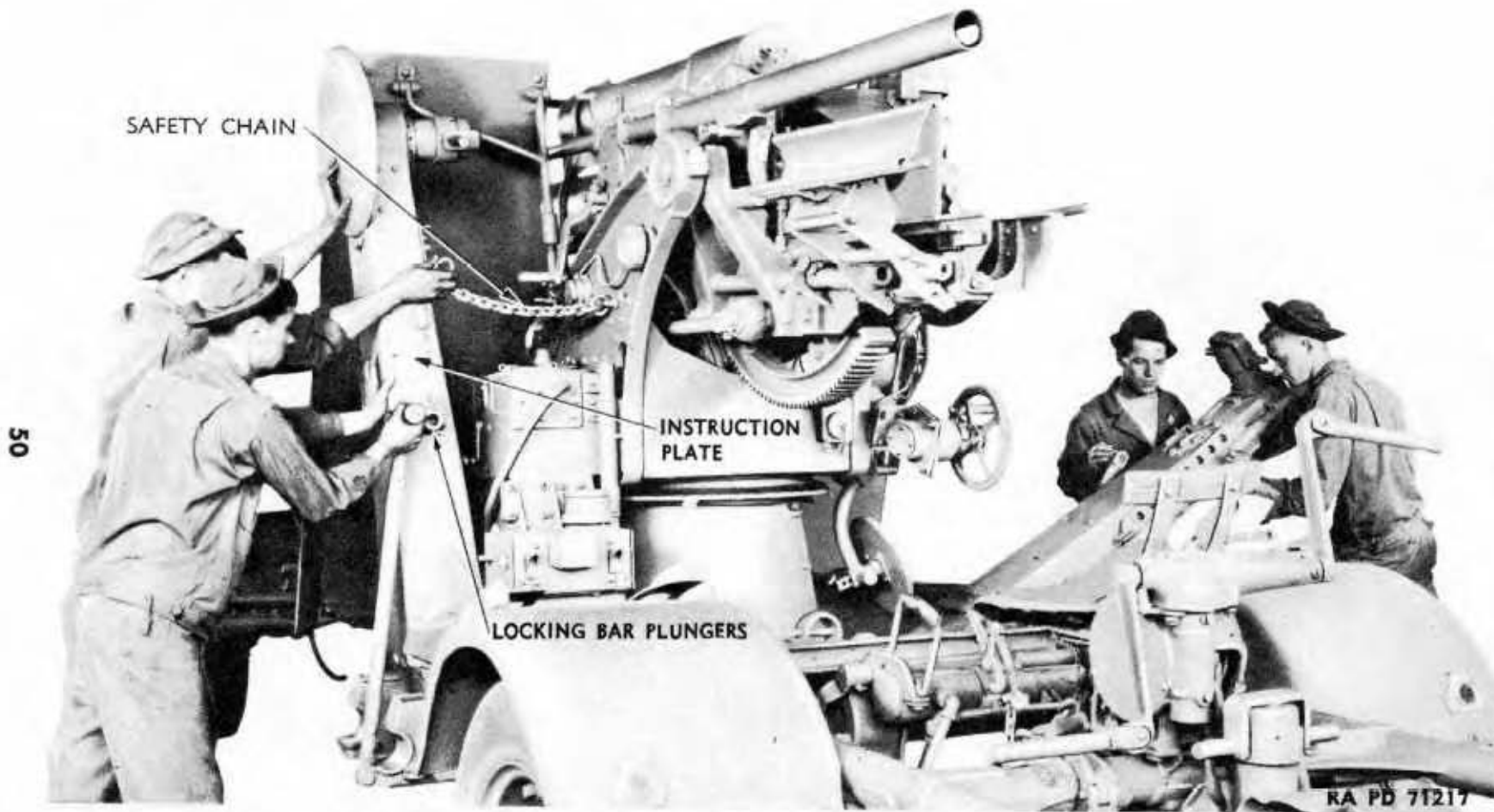
Figure 44 — Releasing Locking Bar Plunger and Removing Safety Chain
