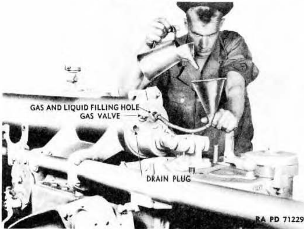
Figure 56 — Filling the Recuperator Cylinder with Liquid
