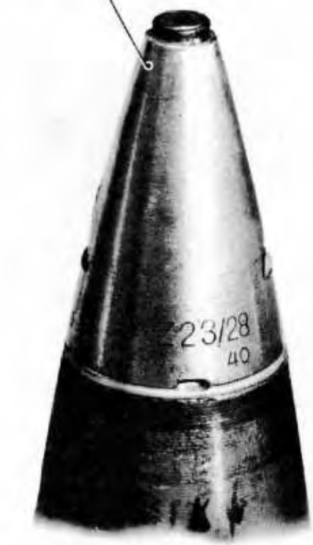
Figure 75 — Spring-wound Time, Percussion, and Inertia-operated Time Fuzes for German 88-mm High-explosive Shell — View Showing Fuze Markings
