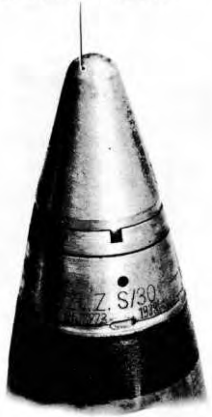
Figure 75 — Spring-wound Time, Percussion, and Inertia-operated Time Fuzes for German 88-mm High-explosive Shell — View Showing Fuze Markings
