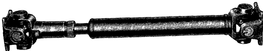
FIGURE 68.—Front axle propeller shaft assembly.
