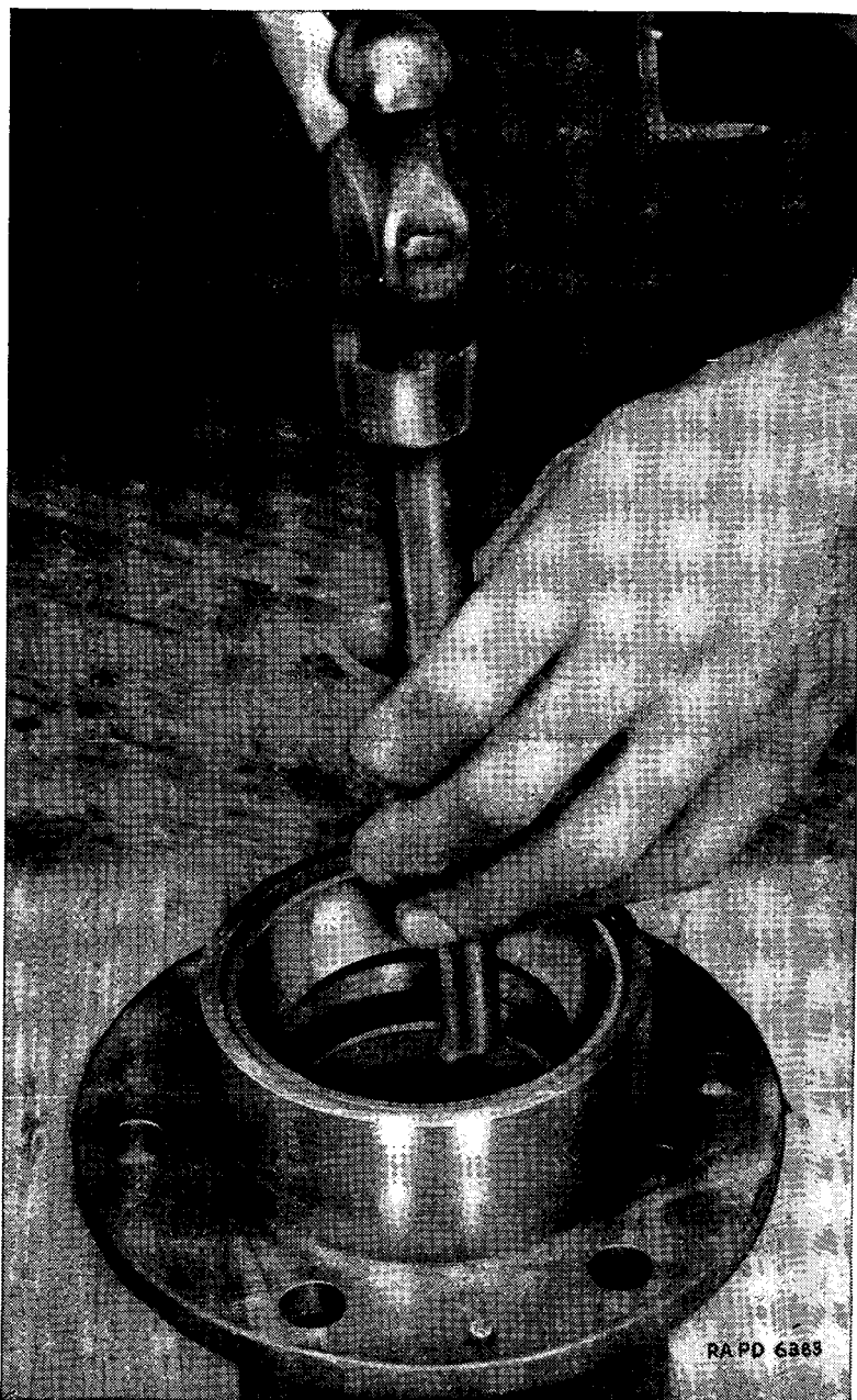
FIGURE 24.—Front axle drive pinion bearing cup removal.
