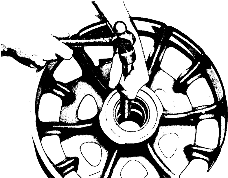
Figure 89 – Inner Bearing and Seal – Removal
