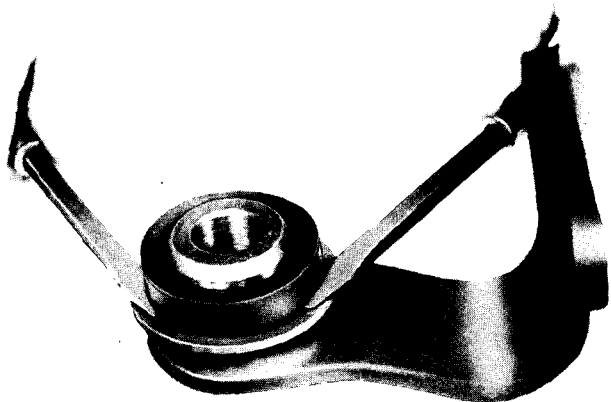
Figure 97 – Upper Roller Seal – Removal
