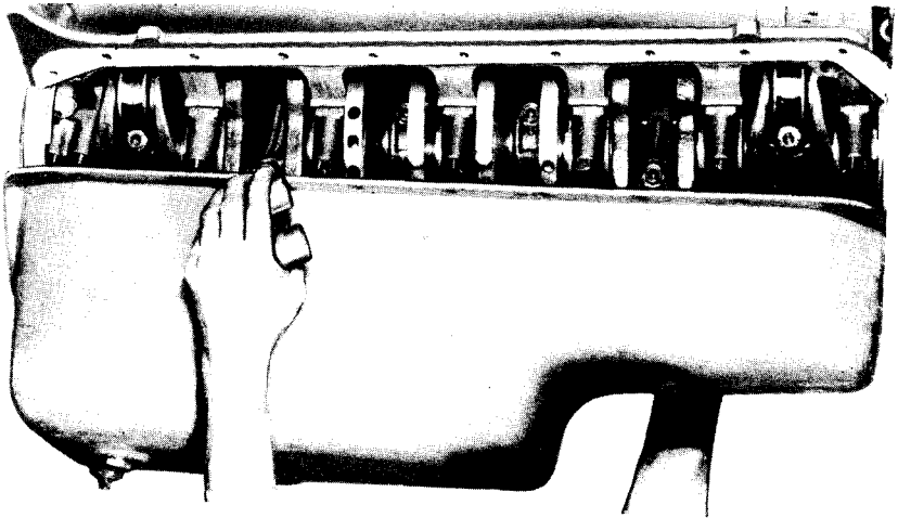
Figure 209 – Oil Pan – Removal
