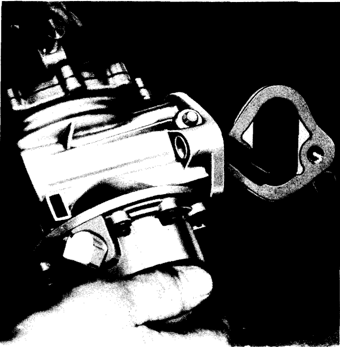
Figure 235 – Fuel Pump – Removal
