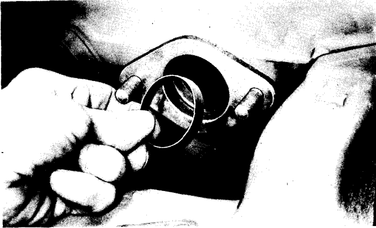
Figure 206 – Intake Manifold Port Seal Rings – Removal
