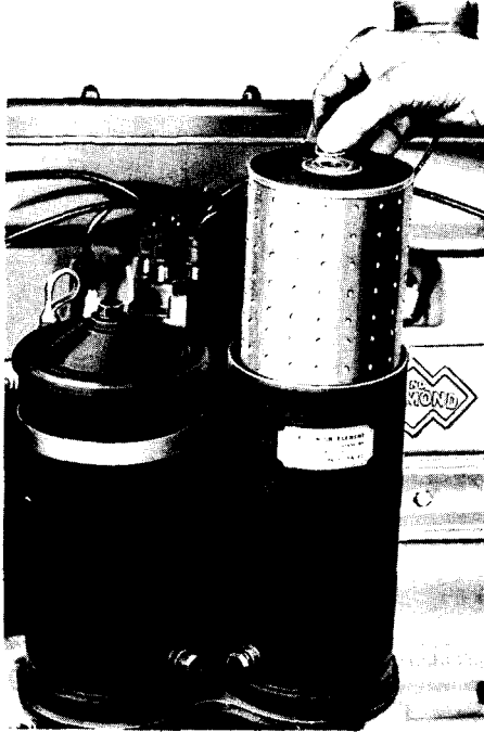
Figure 26 – Oil Filter Cartridge – Installation
