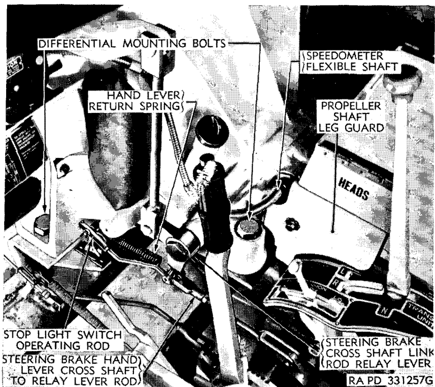
Figure 125. Steering brake linkage and differential mounting.
