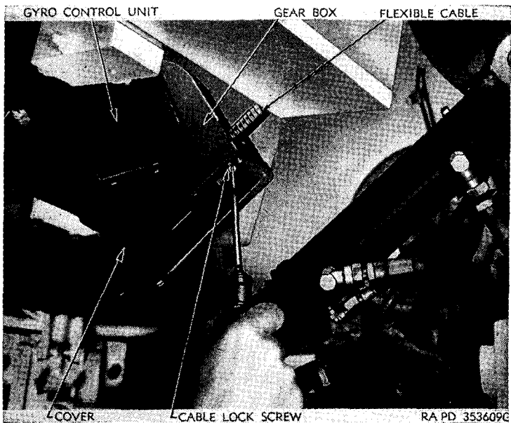
Figure 176. Removing cable from gyro control gear box.
