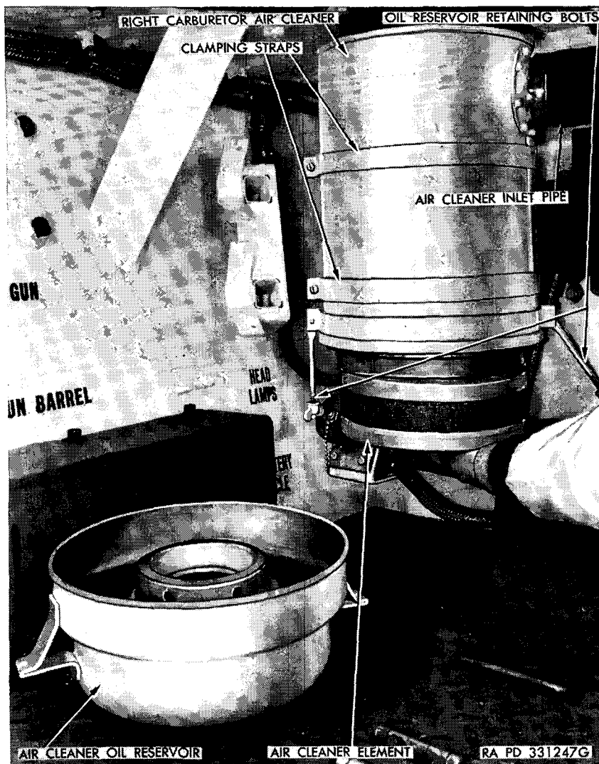
Figure 77. Air cleaner (AC)—servicing cleaner.
