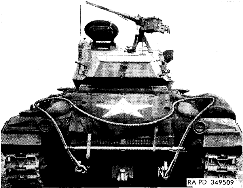
Figure 22. Improvised towing bridle on rear of vehicle.
