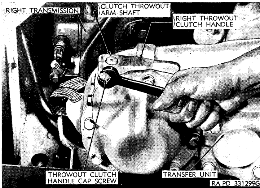
Figure 114. Removing engine input clutch lever.
