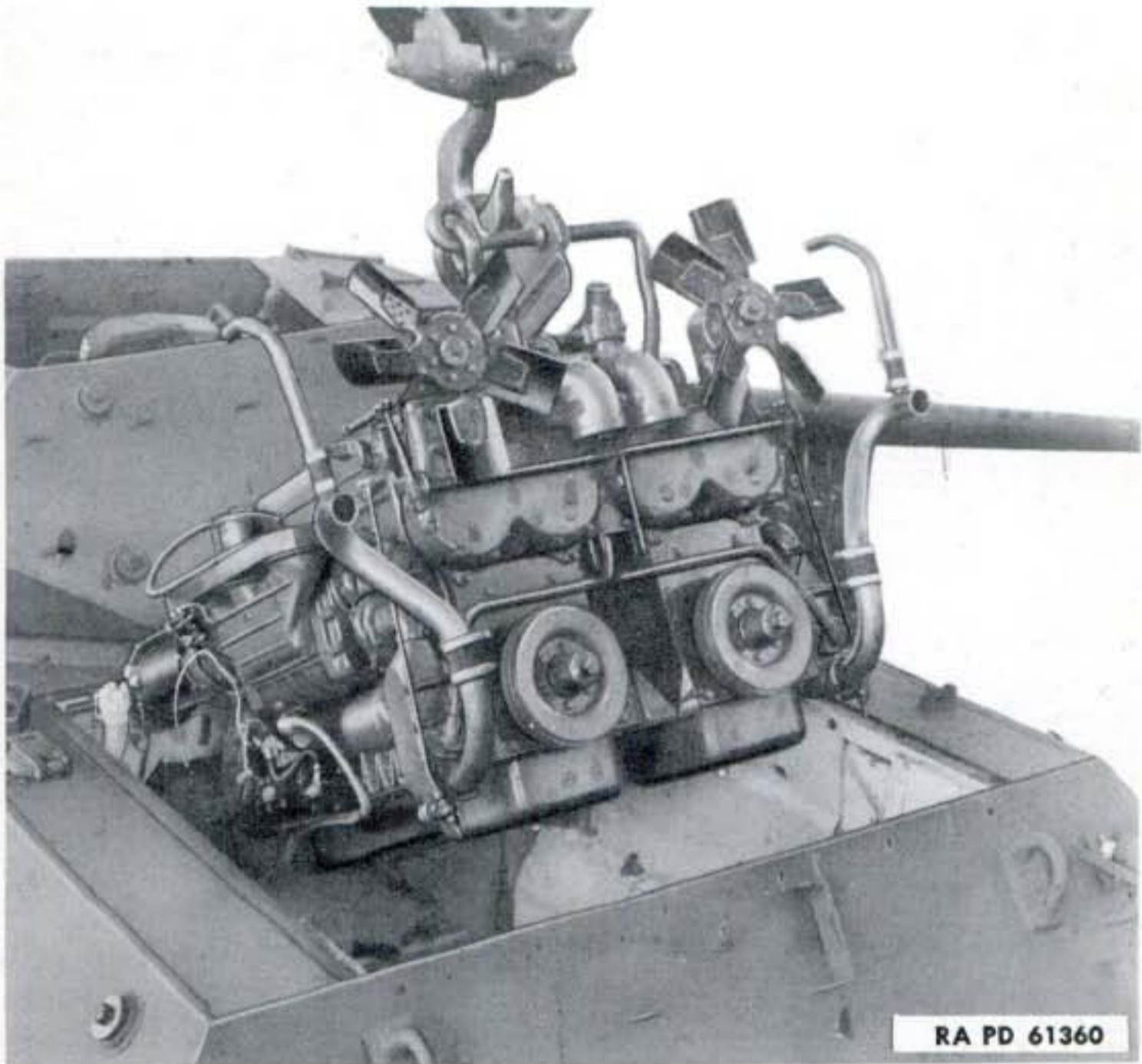
Figure 53—Removing Power Unit from Vehicle—(Engine Lifting Hooks, 41-H-2584)
