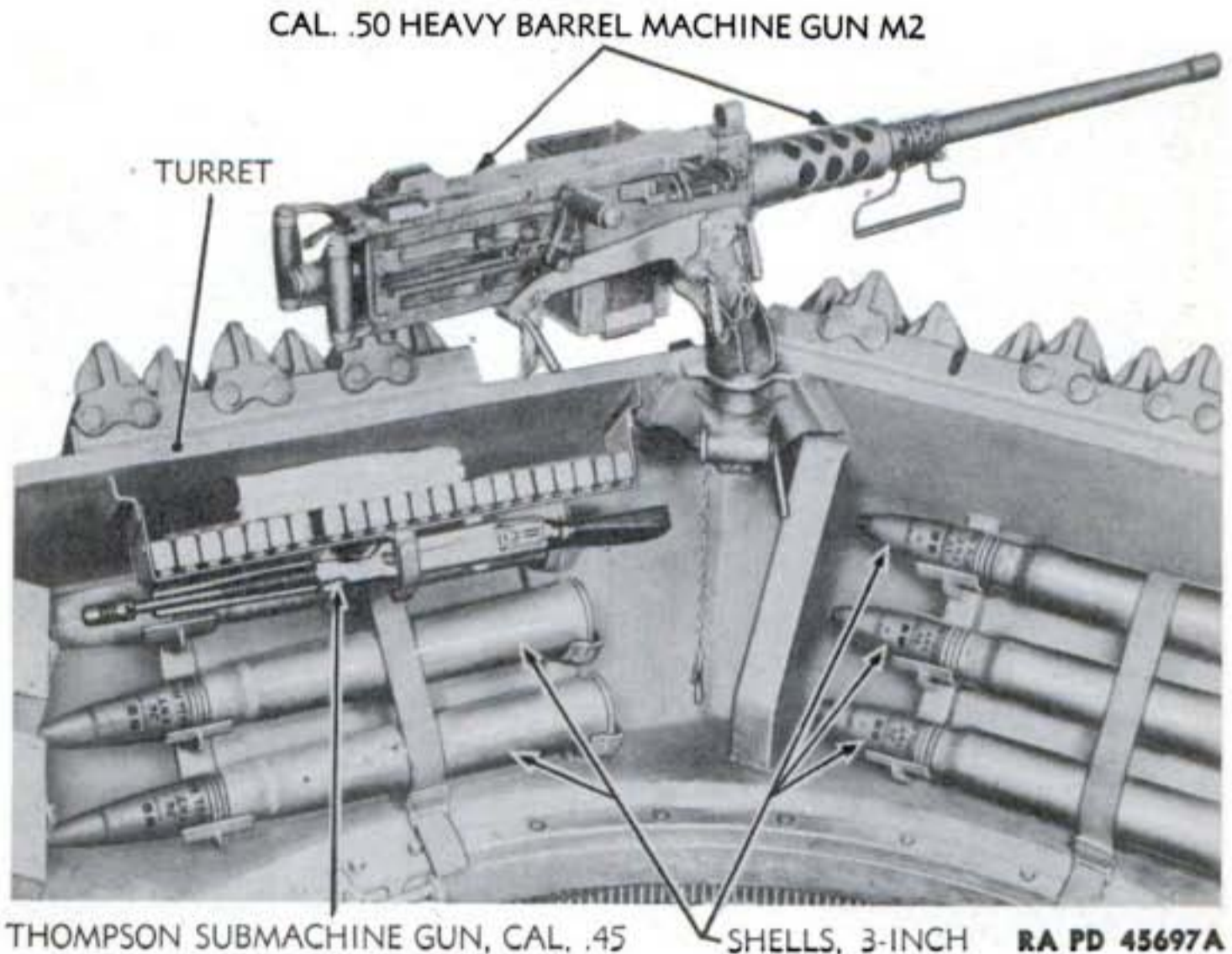
Figure 159—Rear Inside View of Turret
