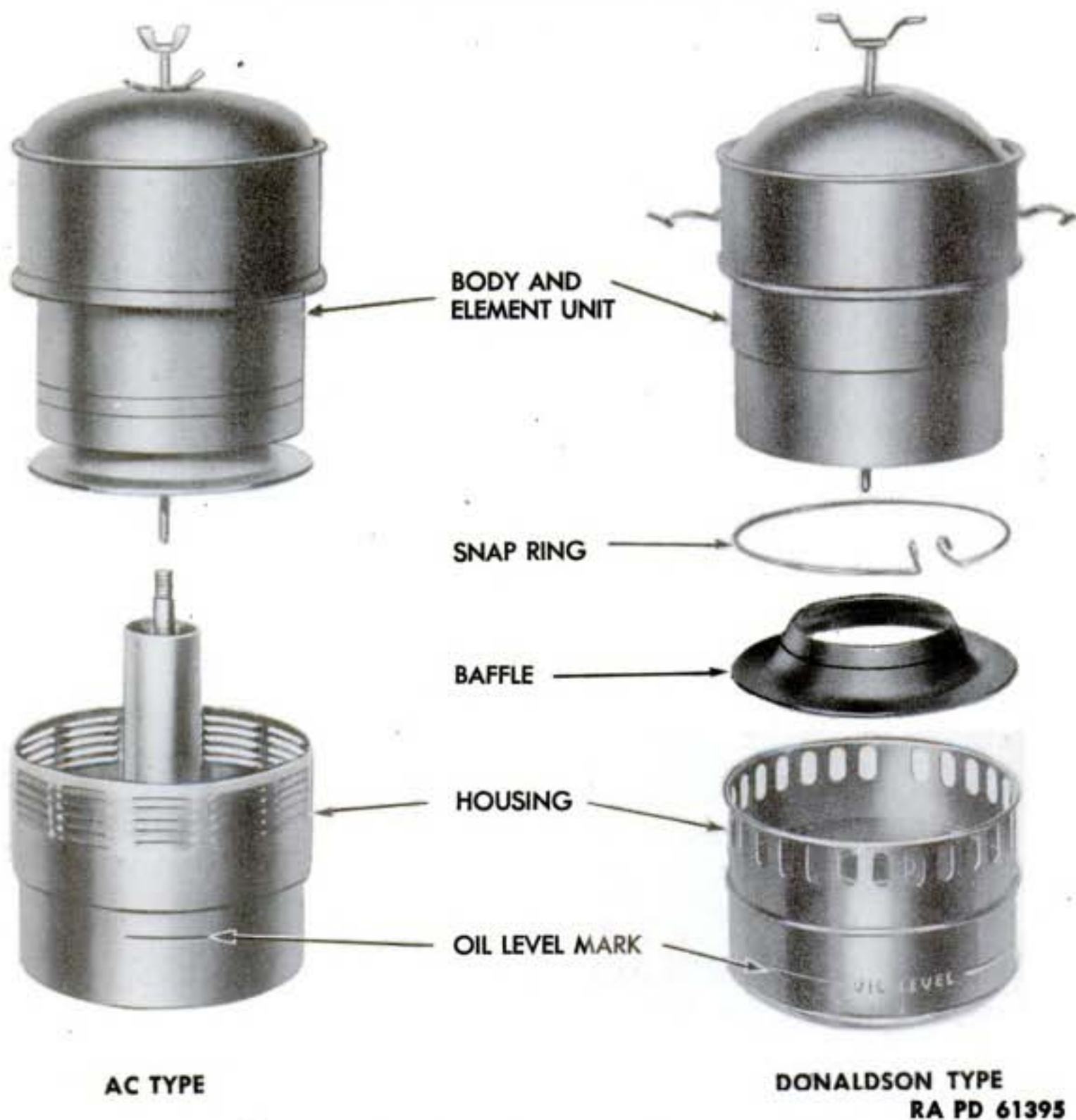
Figure 63—Air Cleaners, Disassembled
