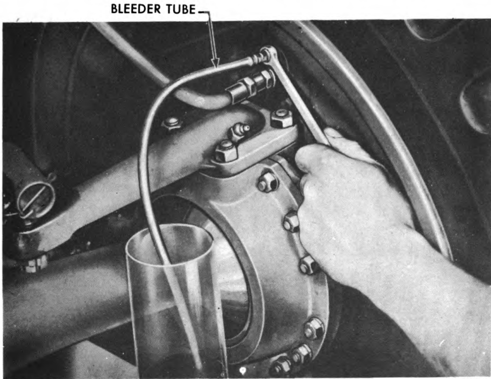
Figure 144—Bleeding Wheel Cylinder RA PD 319216
